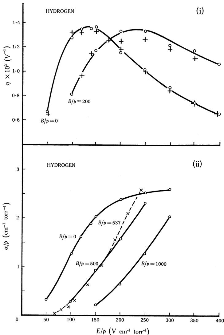
Fig. 3.—(i) Comparison of values of  $\eta$  obtained from measurements made with plane-parallel (+) and coaxial cylindrical (O) geometry in hydrogen for values of  $B/p = 0$  and 200 G/torr; (ii) values of  $\alpha/p$  versus  $E/p$  obtained in the present investigation for  $B/p = 0, 500$ , and 1000 G/torr; also shown for comparison are values obtained by Bernstein (X) corrected to  $0^\circ\text{C}$ .
