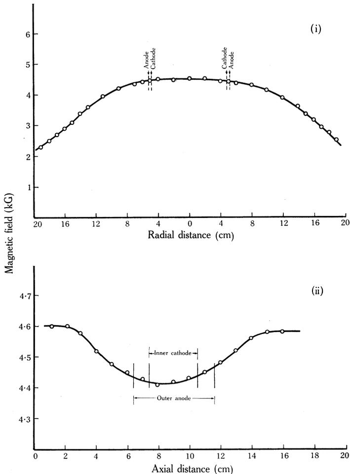
Fig. 2.—Variation of magnetic field between pole faces (i) radially across the magnet air gap in a plane containing the mid point between the two pole faces (also shown is the location of the annular gap, anode-cathode), and (ii) axially across the magnet air gap along a line passing through the ionization region at 5 cm from the axis of symmetry (also shown are the axial lengths of the inner cathode and outer anode).
