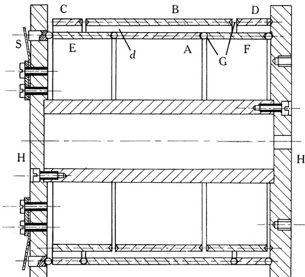
Fig. 1.—Ionization chamber for measurement of gas-amplified currents in  $E \times B$  fields. A, cathode; B, anode; C, D, E, F, guard rings; G, precision-ground  $\frac{1}{8}$  in. sapphire balls; H, non-magnetic stainless steel end plates; S, springs.
