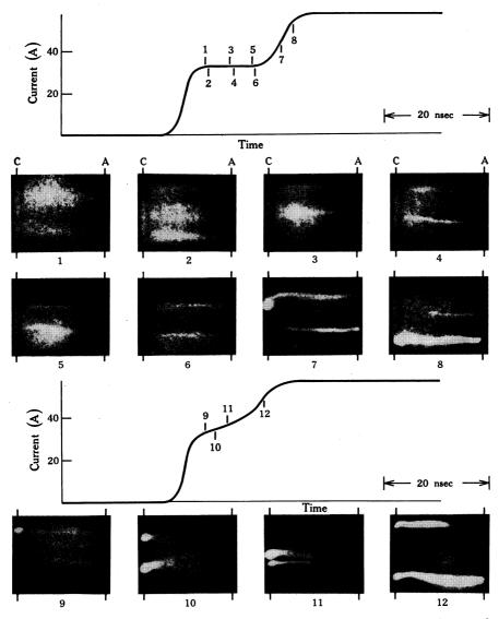
Fig. 2.—Shutter photographs of a discharge in hydrogen at 500 torr and 100% overvoltage (d = 2 mm, V = 5.8 kV).
