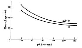
Fig. 1.—Overvoltage required to establish the conditions  $\alpha d = 18$  and 20 as a function of pd.
