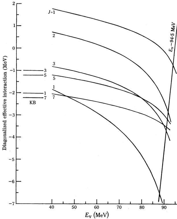
Fig. 2.—Diagonalized effective interaction as a function of the valence energy  $E_v$  for the lowest  $T = 0$  states of  $^{42}\text{Sc}$ . Also shown are the self-consistent line  $E_v - 94.5$  MeV and Kuo and Brown's (1968) diagonalized effective interaction (KB) derived from their bare energy-independent  $G$ -matrix.
