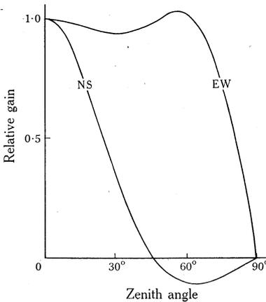
Fig. 1.—Calculated north-south field patterns of the north-south (NS) and east-west (EW) arrays.
