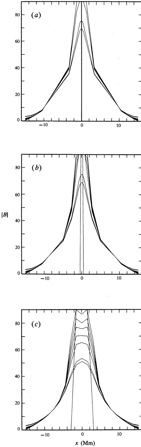
**Fig. 3.** Absolute field strength against horizontal position at several heights. Cell diameter and mean field are as in Fig. 2. Network widths are (a) 0.05 Mm; (b) 0.5 Mm; (c) 5.0 Mm.
