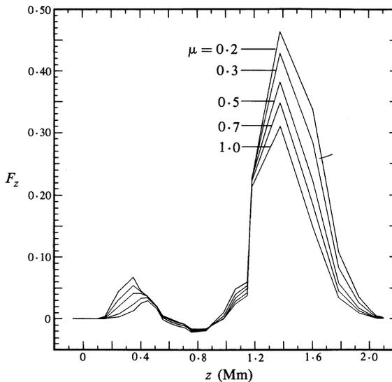
Fig. 1. Response function  $F_z$  for depth-varying magnetic fields for the 8542 Å line of Ca II in the VAL model C atmosphere at various values of  $\mu$ . Wavelength integration and normalization are appropriate for the NSO/Tucson Vacuum Telescope with the 'synoptic' exit slit (see Section 3 for further discussion).
