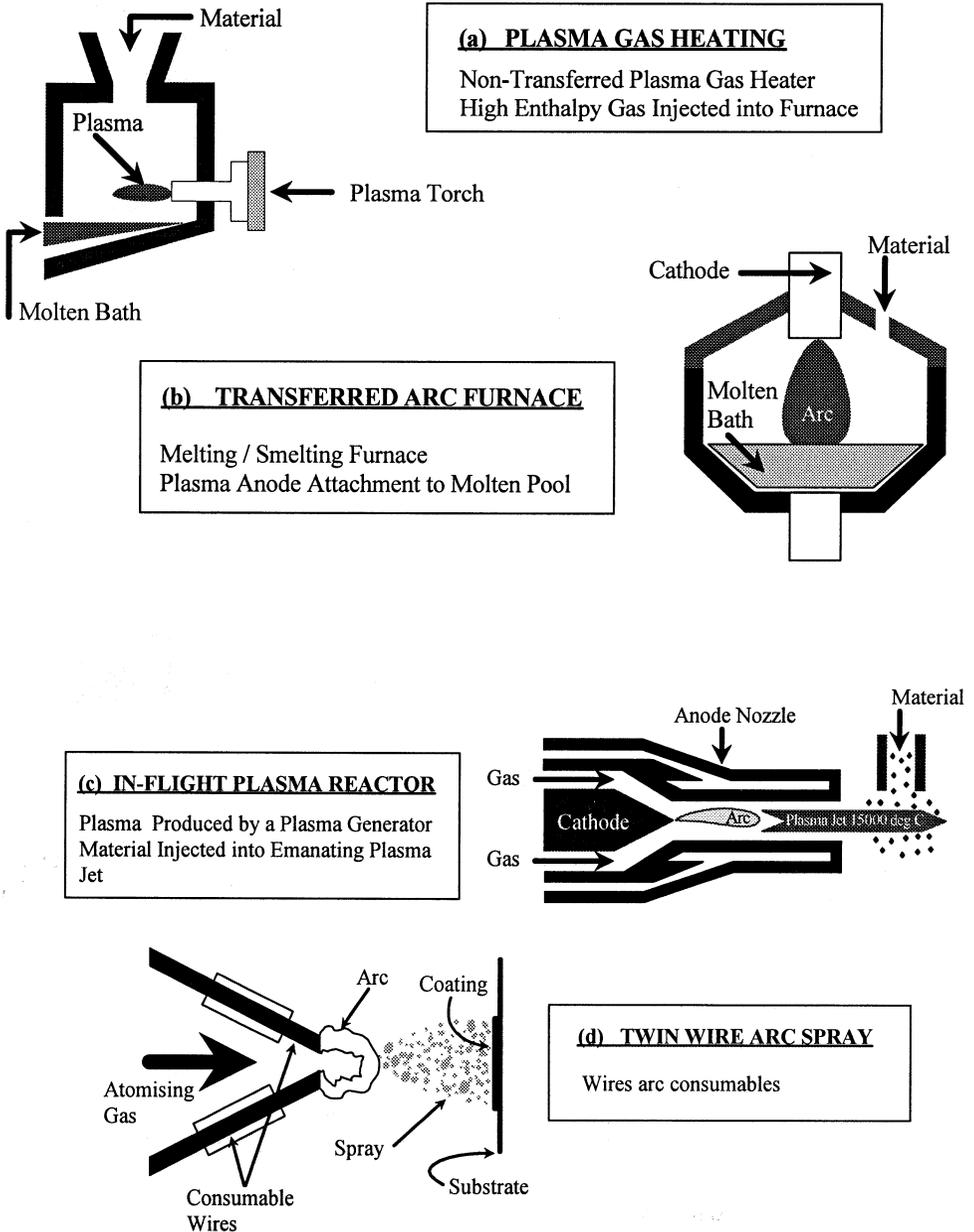
Fig. 2. Configurations of plasma/arc processors.
