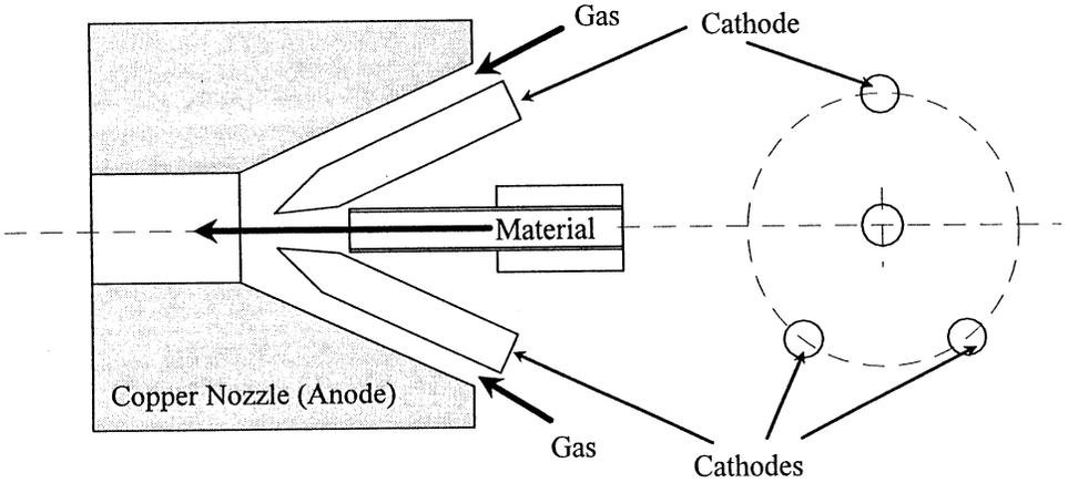
Fig. 9. Plasma torch with three cathodes for axial material injection.
