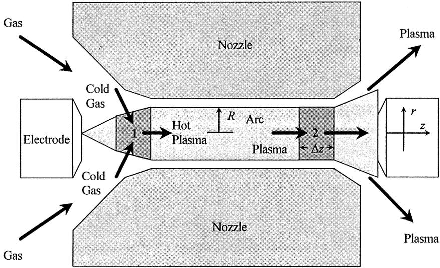
Fig. 7. An electric arc in forced convection.
