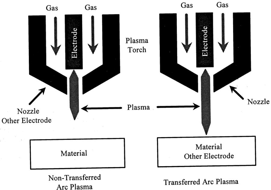
Fig. 1. Transferred and non-transferred plasmas.
