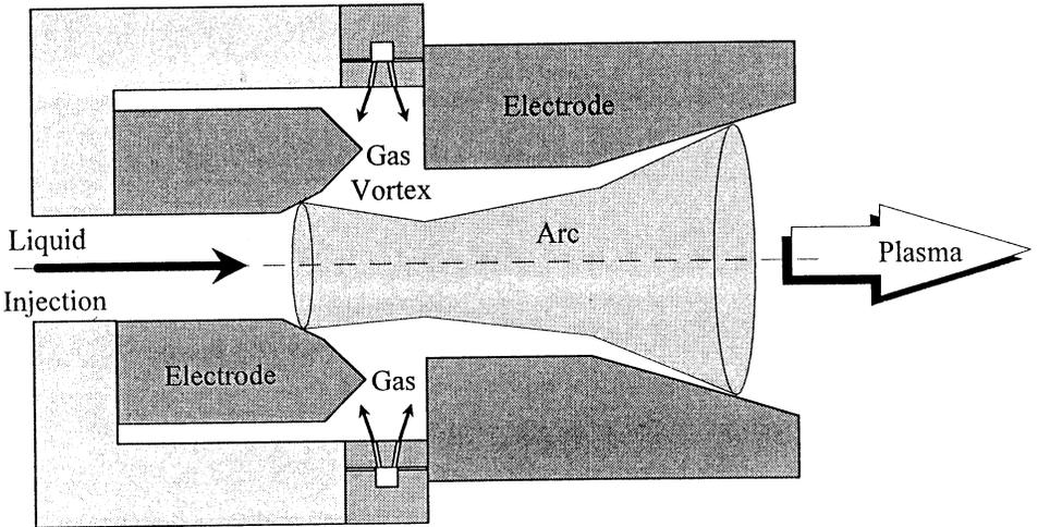
Fig. 10. The Tiddalik plasma reactor for axial injection of material.
