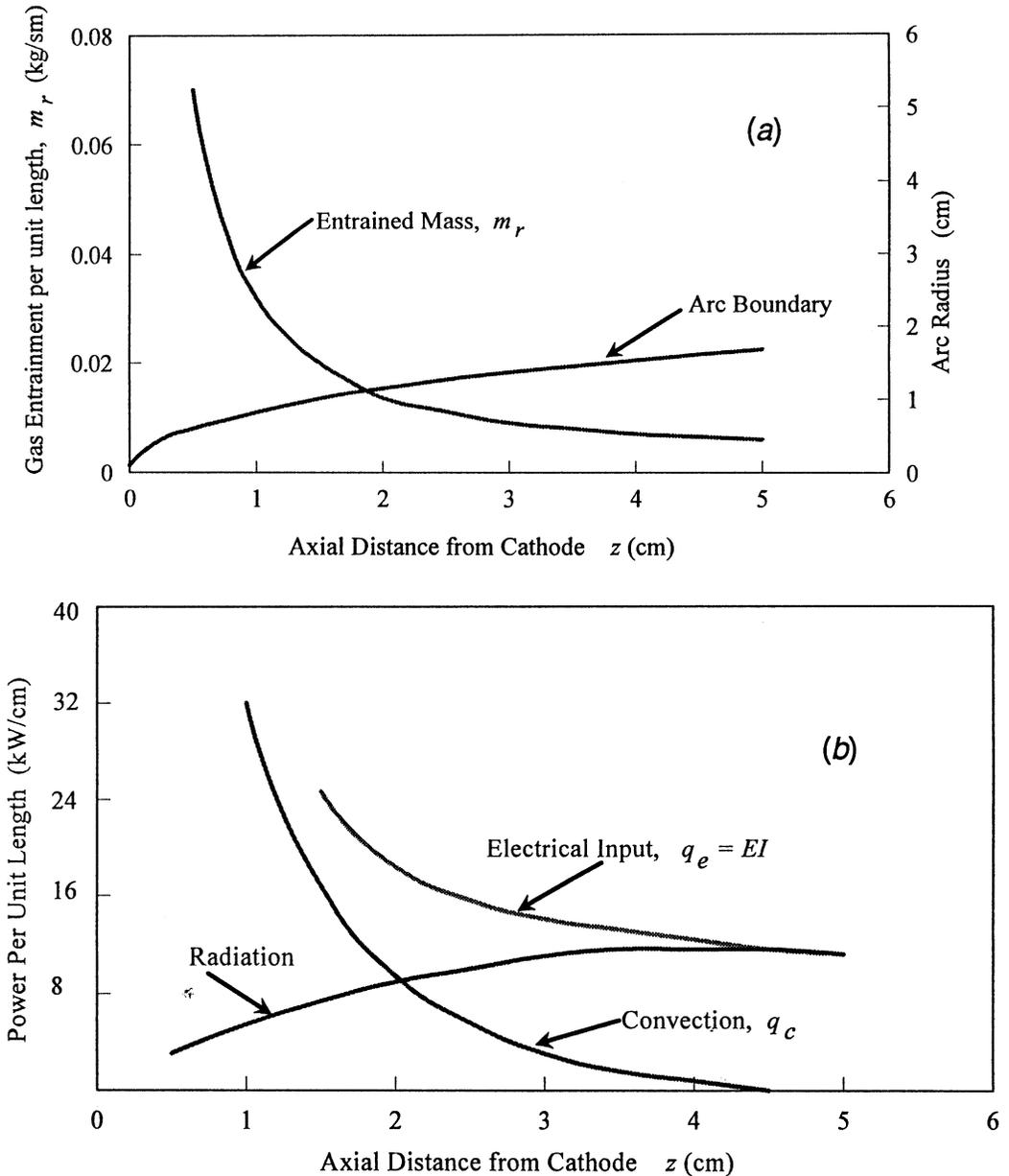
Fig. 8. Properties of a 2.16 kA free-burning arc in air with induced gas flows near the cathode.
