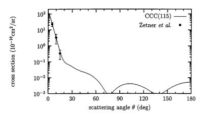
Fig. 8. Differential cross section for electron scattering from the  $6s5d^1D_2^e$  to the  $6s7p^1P_1^o$  state of barium (Moore's label:  $6p5d^1P_1^o$ ) at 20 eV. Experimental data are by Zetner *et al.* (1999).
