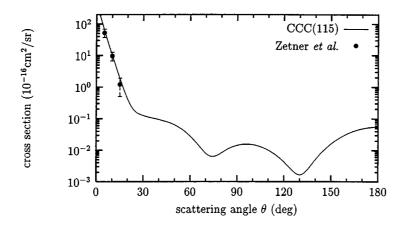
Fig. 9. Differential cross section for electron scattering from  $6s5d^3D_2^e$  to the  $6p5d^3P_{1,2}^o$  states of barium at 20 eV. Experimental data are by Zetner *et al.* (1999).
