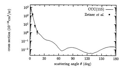
**Fig. 6.** Differential cross section for electron scattering from the  $6s6p^1P_1^o$  to the  $6s6d^1D_2^o$  state of barium at 20 eV. Experimental data are by Zetner *et al.* (1997).
