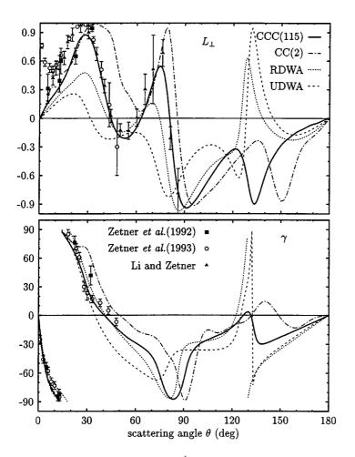
**Fig. 3.** EICPs  $L_{\perp}$  and  $\gamma$  of the  $6s6p^1P_1^{\circ}$  state for electron scattering on the Ba ground state at 20 eV. Theoretical calculations are as for Fig. 2. Measurements are by Zetner *et al.* (1992, 1993) and Li and Zetner (1994).
