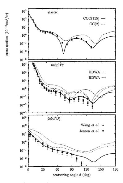
**Fig. 2.** Elastic,  $686p^1P_1^{\circ}$  and  $685d^1D_2^{\circ}$  excitation differential cross sections for electron scattering from the Ba ground state at 20 eV incident electron energy. The CCC(115) calculation is described in the text. The UDWA calculations are due to Clark *et al.* (1989), the RDWA calculations are due to Srivastava *et al.* (1992*a*, 1992*b*) and the CC(2) calculations are due to Fabrikant (1980). Measurements are by Wang *et al.* (1994) and Jensen *et al.* (1978).
