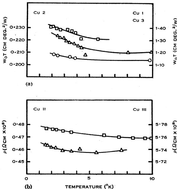
Fig. 4.—Residual resistance of copper below 10 °K. (a) The product of the residual thermal resistance and temperature,
