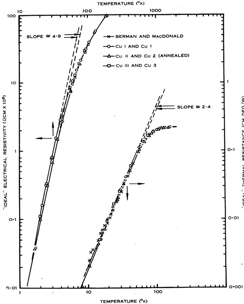
Fig. 3.—“Ideal” electrical and thermal resistance of copper.
