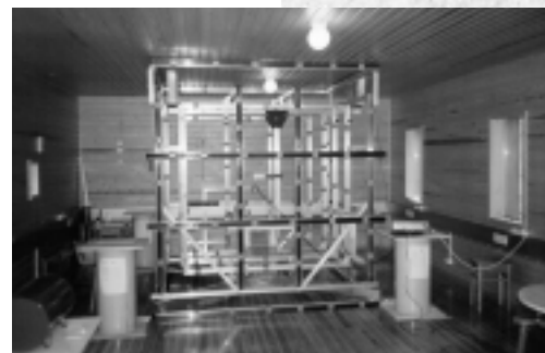
The picture shows the Finnish calibration coil system. This comprises of four sets of copper windings on each of the three orthogonal axes. The frame is made of aluminium.
