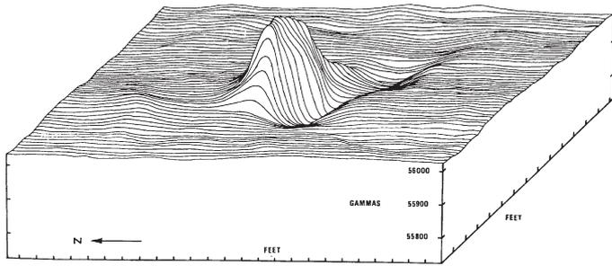
**Figure 3.** A pseudo isometric image of the magnetic field recorded over a fire hearth that had been left burning for 24 hours. The image was produced by tracing analogue profiles automatically plotted during data acquisition, each with a scaled offset from the front of the image to the back. (1 gamma = 1 nT).
