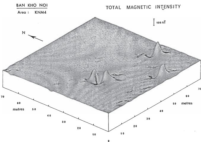
**Figure 8.** The magnetic field mapped in Thailand in 1984 with a TM-2 magnetometer. The four anomalies visible indicate the location of four pottery kilns from the Sukhothai period of 1250 to 1500 AD.
