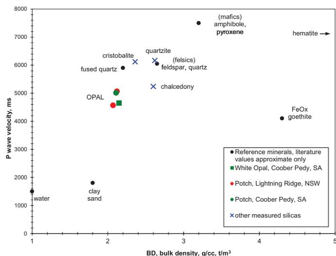
**Figure 6.** A plot of compressional (P) wave ultrasonic velocity (100 kHz) against bulk density for common opal samples. The data are referenced to a notional weathered environment mineralogy. There are distinct differences in velocity and density between the opaline silicas and quartz.
