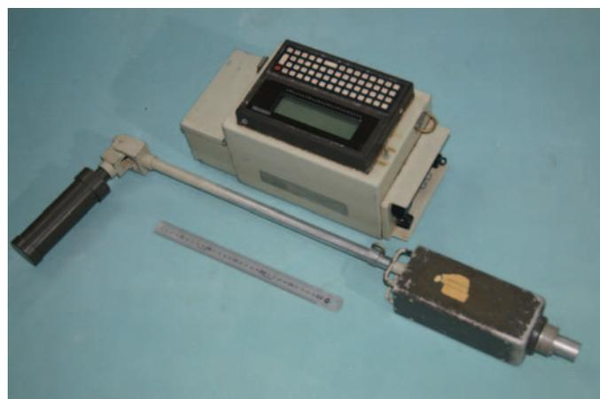
**Figure 11.** The TM-3 magnetometer with microprocessor controlled survey management aids, inbuilt odometer and digital recording from up to two optically pumped sensors.
