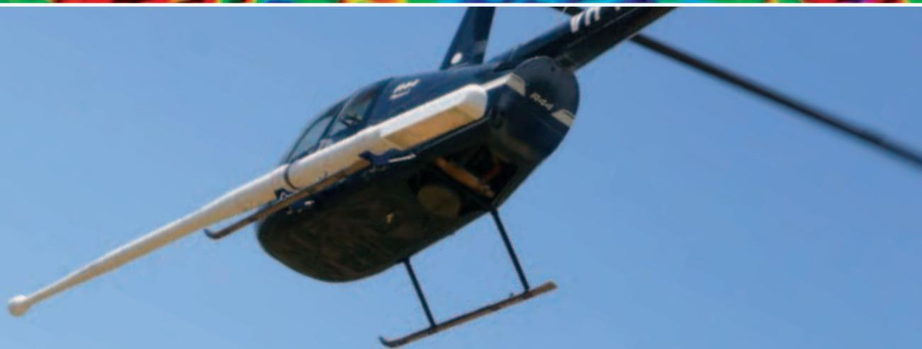
World first piston engine helicopter stinger installation for low cost, high quality airborne radiometric and magnetic data collection
