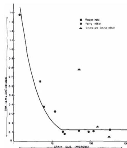
**Figure 2.** Dickson et al.'s Fig. 1 combining Roquet's (1954), Parry's (1965) and Ozima and Ozima's (1965) thermoremanent magnetisation (TRM) vs grain-size results showing the abrupt onset of multidomain behaviour above 20  $\mu\text{m}$  where TRM is no longer a function of grain-size or coercivity.
