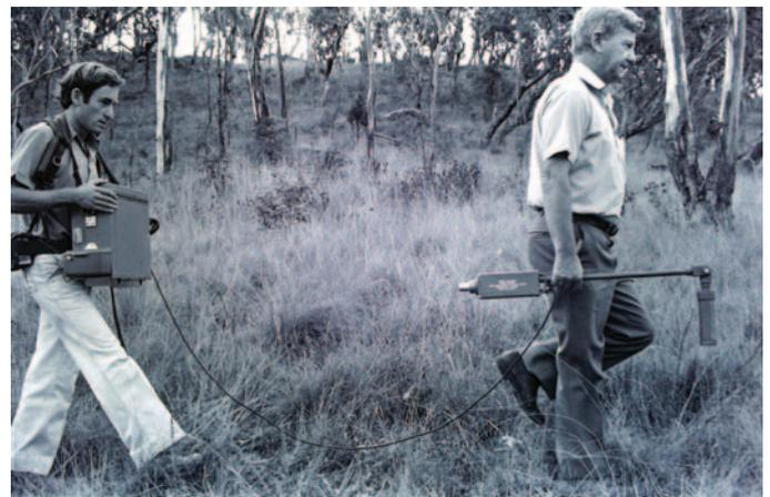
**Figure 6.** The 'telemetric magnetometer' TM-1 encoded digital data in an audio code suitable for transmitting by CB radio to the vehicle-borne digital data acquisition system. With the advent of the Sony Walkman cassette recorder in 1979, the troublesome CB link was replaced. The instrument shown here was the first portable magnetometer with inbuilt memory and a data positioning device.
