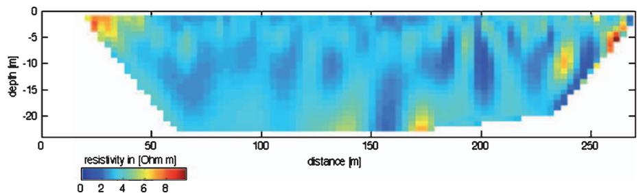
**Figure 2.** 2D electrical resistivity inversion, Leque Island Washington, USA, 2013. The electrical resistivity measurements are dominated by the conductivity of the groundwater below 5 m, and hence indicate little variability below 5 m.
