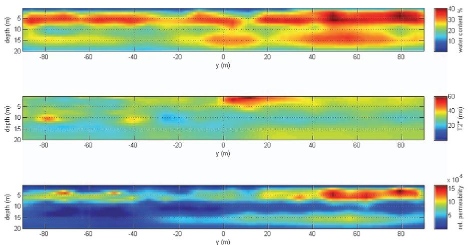
**Figure 3.** 2D surface NMR inversion, Leque Island Washington, USA, 2013. The 2D surface NMR inversion clearly indicates the presence of a laterally continuous upper aquifer at a depth of about 5 m, and a laterally discontinuous aquifer at a depth of about 15 m.
