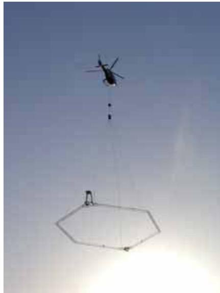
Fig. 2. The SkyTEM system configuration.
