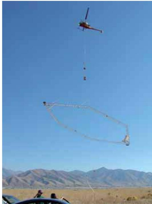
Fig.1. The SkyTEM system in operation, Utah, October 2005.
