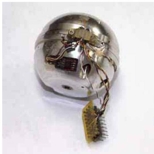
Fig. 1. Scintrex BH gravity sensor ball. It is about the size of a ping pong ball.
