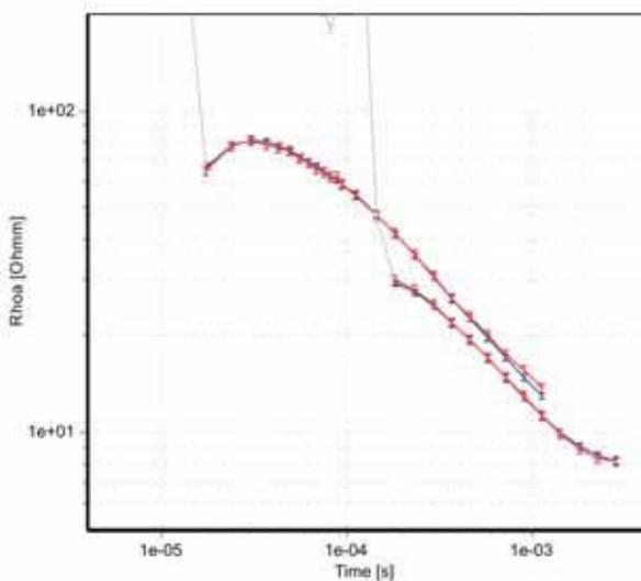
Fig. 3. Example of verification check of the SkyTEM system versus ground based TEM data. The blue curve represents ground based data upward continued to 10 m height. The red curve indicates actual SkyTEM data acquired at a height of 10 m. The error between the data sets ranges from 2% - 3%. The SkyTEM data has not had drift or system response corrections applied.
