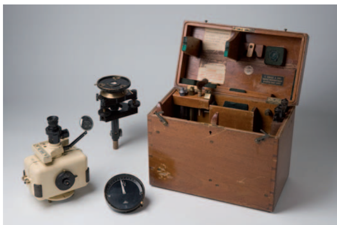
Fig. 13. Watts variometer no. 15887. Image: National Museum of Australia, 2007.
