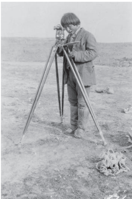
Fig. 8. Took-a-key viewing the azimuth mark with theodolite-magnetometer CIW-16 at Cape Dorset, Baffin Land, August 1922. Image: Carnegie Institution of Washington, Department of Terrestrial Magnetism, 2013.
