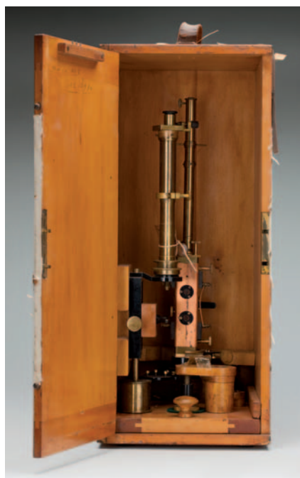
Fig. 6. Toepfer mirror galvanometer no. 2. Image: National Museum of Australia, 2013.
