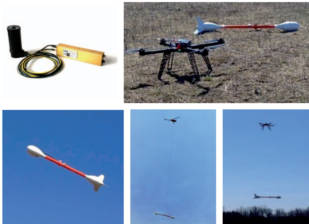
Figure 1. Sling-mounted magnetometer weighing ~3.3 kg hanging under various UAVs. The system's heart is the Gem GSMP 35U Potassium UAV magnetometer shown in the upper left ( www.gemsys.ca/uavs-pathway-to-the-future/ ).
