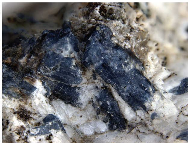
Figure 10: Bluish-grey schorl–elbaite crystals up to 4 mm long from the Klocker pegmatite. Museum Victoria M51168. Photographer Simon Hinkley.
