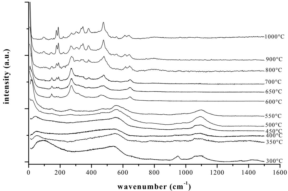
Figure 1: Waveguide Raman spectra for  $\text{ZrO}_2$  at varying annealing temperatures.
