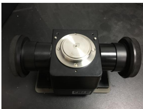
Fig. S1. The single-reflection diamond ATR unit (Pike Technologies, Inc.; Part No. is P025-2100).
