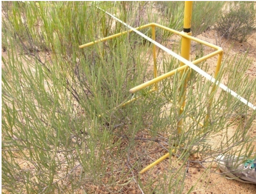
Fig. S1. Cubic fuel sampler for collection of fuel at each 25 cm level. Fuel was removed from within the frame, and was bagged for drying and weighing. (Source: S. Dalglish)
