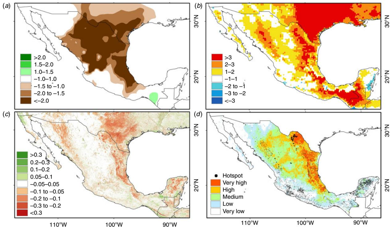
**Fig. 4.** Climatic hazards during April 2011: (a) SPI-3; (b) surface temperature anomaly ( $^{\circ}\text{C}$ ); (c) Normalized Difference Vegetation Index (NDVI) anomaly; and (d) ranks of the resulting climate hazard index. Black dots indicate fires detected by satellite.
