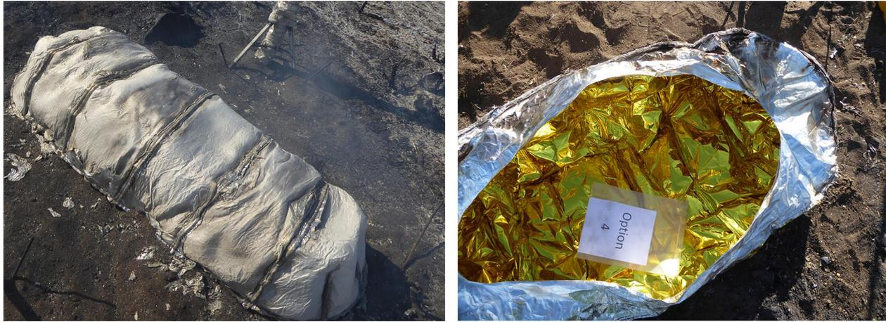
**Fig. 4.** Photo of Prototype 4 in Field Test 1. Left shows 99% exterior damage and right shows interior free of damage.
