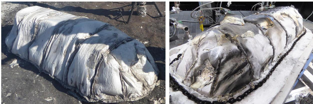
**Fig. 7.** Photo comparing shelter degradation in field burn (left), and in PyroDome™ test (right).
