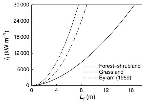
**Fig. 4.** Graphical representation of Byram's (1959) fireline intensity ( $I_f$ )–flame length ( $L_f$ ) relationship ( $I_f = 259.8 L_f^{2.174}$ ) and the corresponding models developed in the present study (Table 2).
