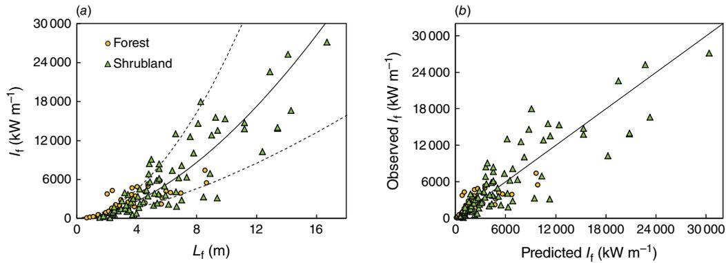
**Fig. 2.** Eqn 2 fit and evaluation for forest–shrubland after back transformation: (a) Fireline intensity ( $I_f$ ) as a function of flame length ( $L_f$ ), dashed lines are the 95% CI; and (b) observed vs predicted  $I_f$  values. Fitted coefficients and evaluation metrics are given in Table 2.
