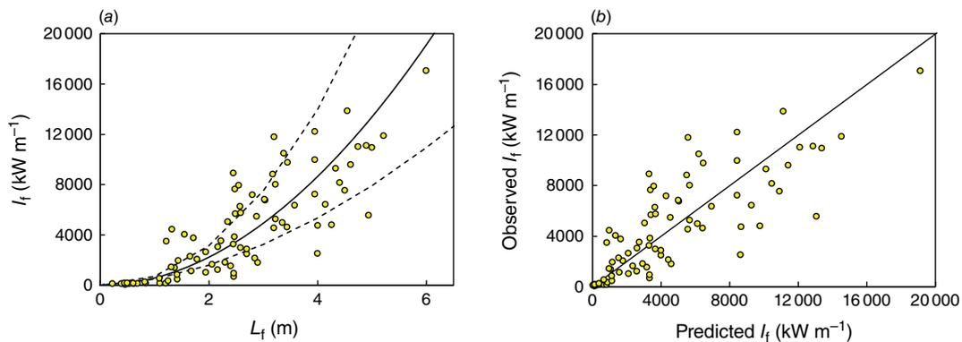
**Fig. 3.** Eqn 2 fit and evaluation for grassland after back-transformation: (a) Fireline intensity ( $I_f$ ) as a function of flame length ( $L_f$ ), dashed lines are the 95% CI; and (b) observed vs predicted  $I_f$  values. Fitted coefficients and evaluation metrics are given in Table 2.
