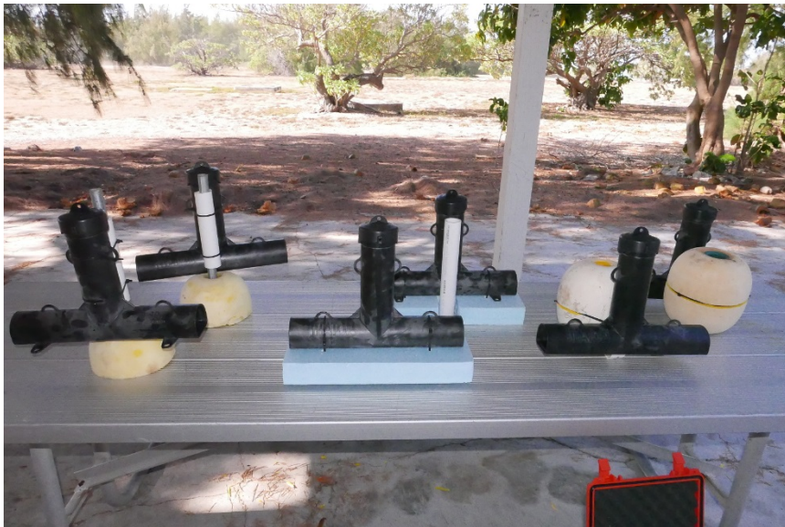
Fig. S6. Floating bait station prototypes. Left: Standard box-type bait station with hole cut through center positioned over EMT center pole. Right: Variations on a T-type floating bait station, also to be sheathed onto an EMT center pole. Photos: S. Siers.
