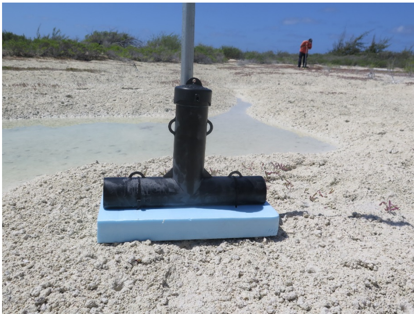
Fig. S5. Floating bait station designs. Left: bait station on a free-floating platform tethered to a stake. Right: Bait station on a foam platform with a tube collar, free to float up and down with the tide along the metal center pole. Photos: S. Siers.
