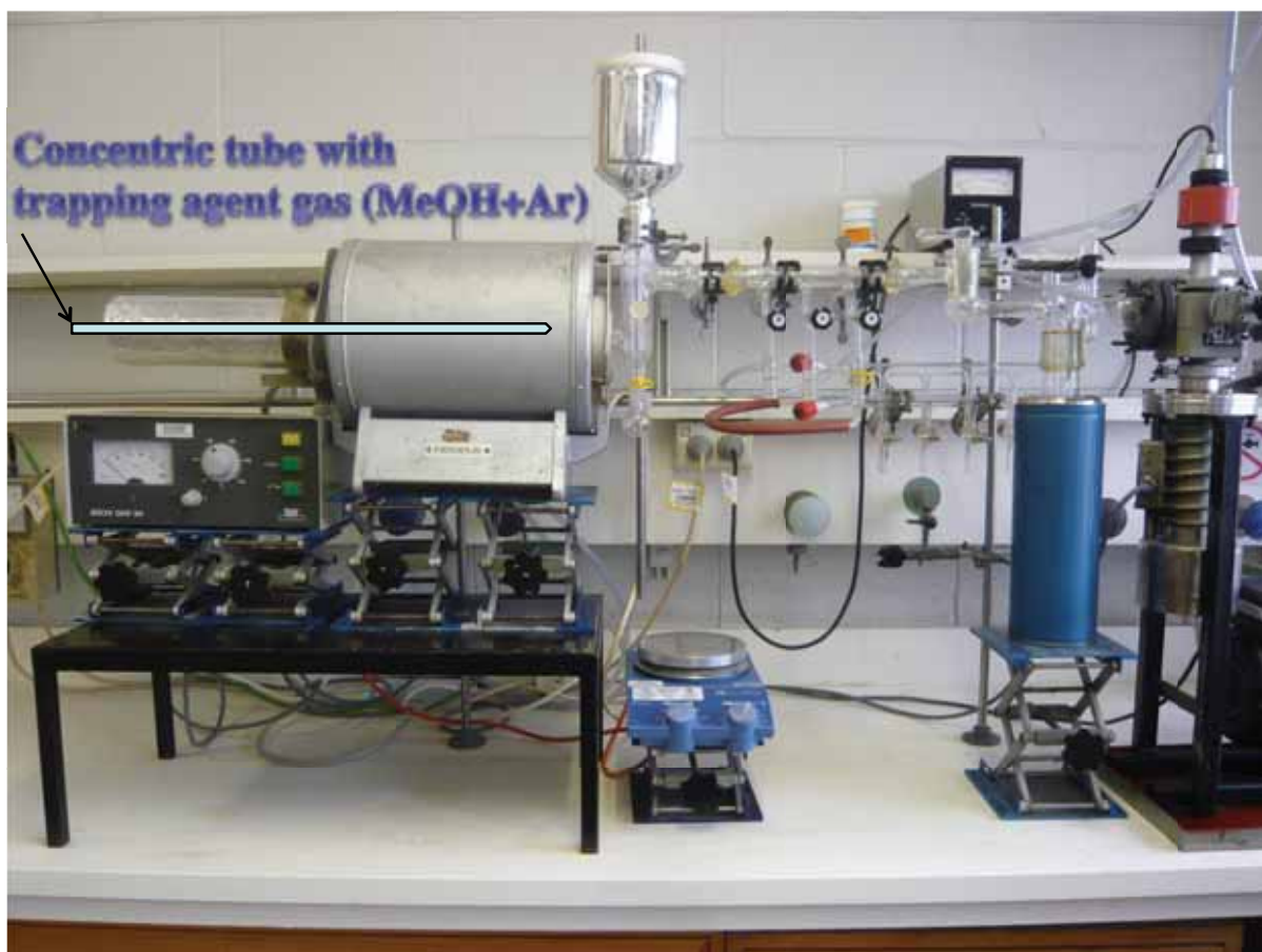
Figure S3. Schematic illustration of concentric tube trapping of reactive molecules (“hot trapping”). For example, the three individual ketenes in Figure S4 may be trapped, e.g. with MeOH. The inner, concentric, tube (2-4 mm I.D.) passes through the sample inlet tube and the pyrolysis tube (20 mm I.D.) and terminates near the end of the pyrolysis tube (the exact length can be varied) (see Figure S2). Ar or N 2 is used as a carrier gas to minimize back-streaming of trapped product. A premixed mixture of trapping agent and carrier gas is fed in through a needle valve or a capillary, or the trapping agent is entrained by the stream of carrier gas. For small scale work the mixture of trapped product and excess trapping agent is collected on the cold finger (77 K), and for larger scale work better in one or two consecutive cold traps.
