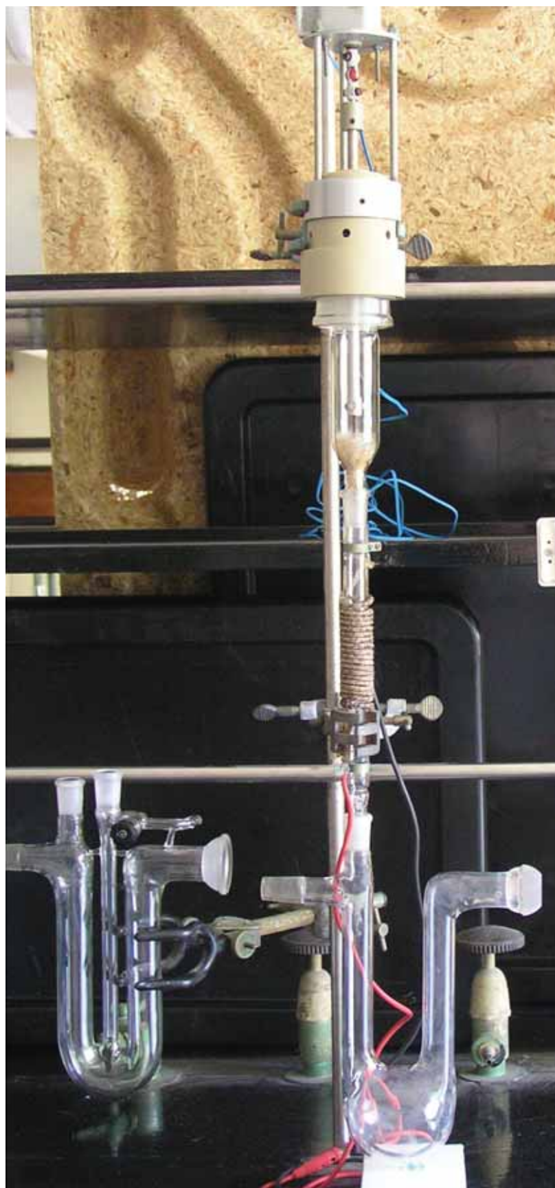
Figure S5. A simplified version of the piptopysolysis apparatus. Photo by the author.
