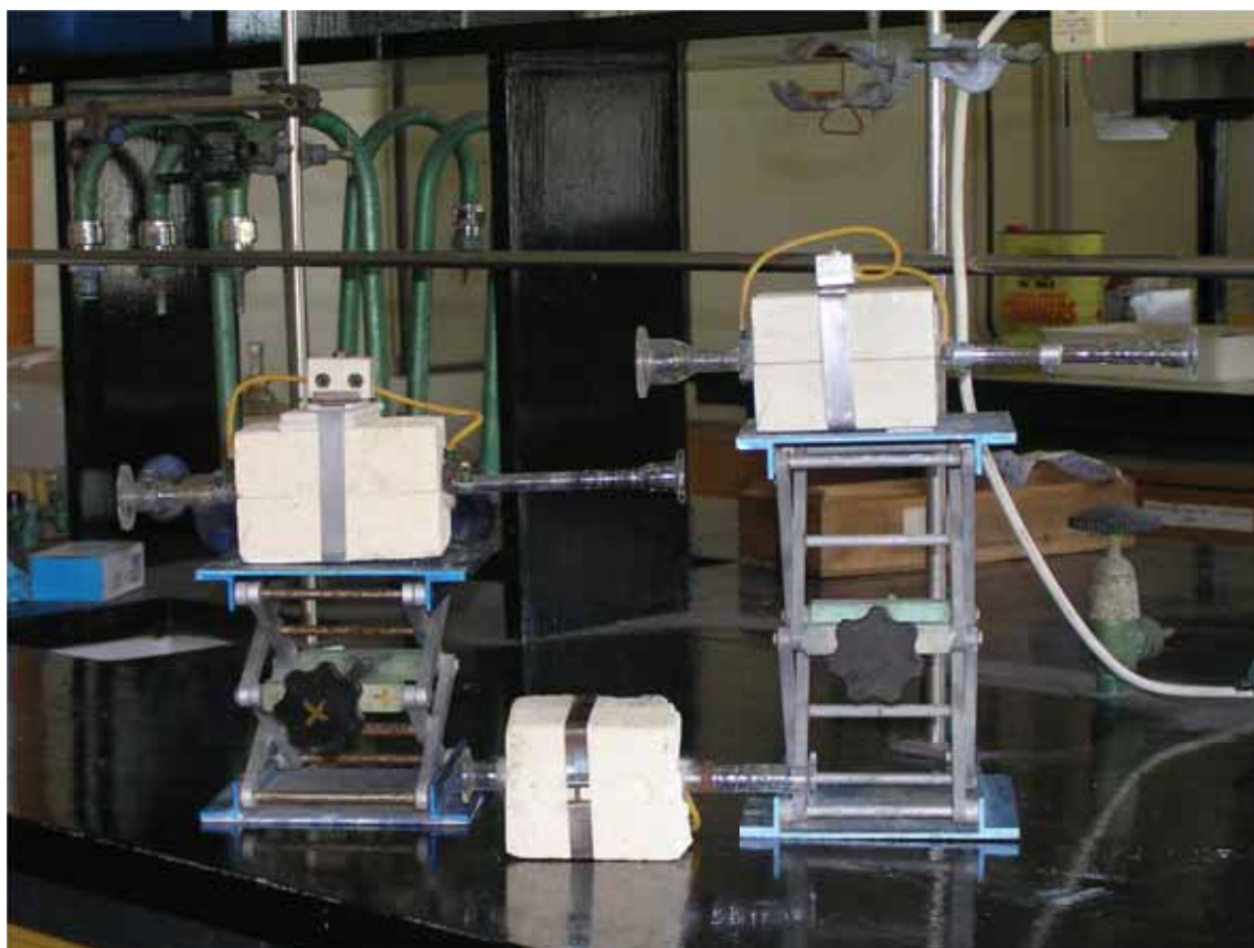
Figure S11. Three types of “brick” pyrolyzer tubes (cf. Figure 10 in the paper proper).
