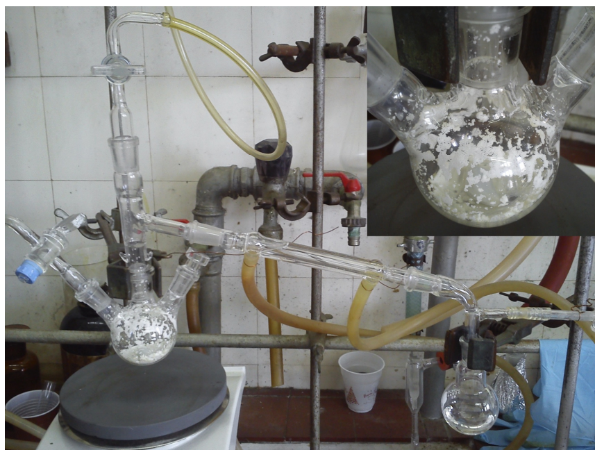
Figure SM1. The apparatus for toluene distillation under an argon atmosphere. Inset: a close-up view of the Vilsmeier salt 2 after removing toluene.
