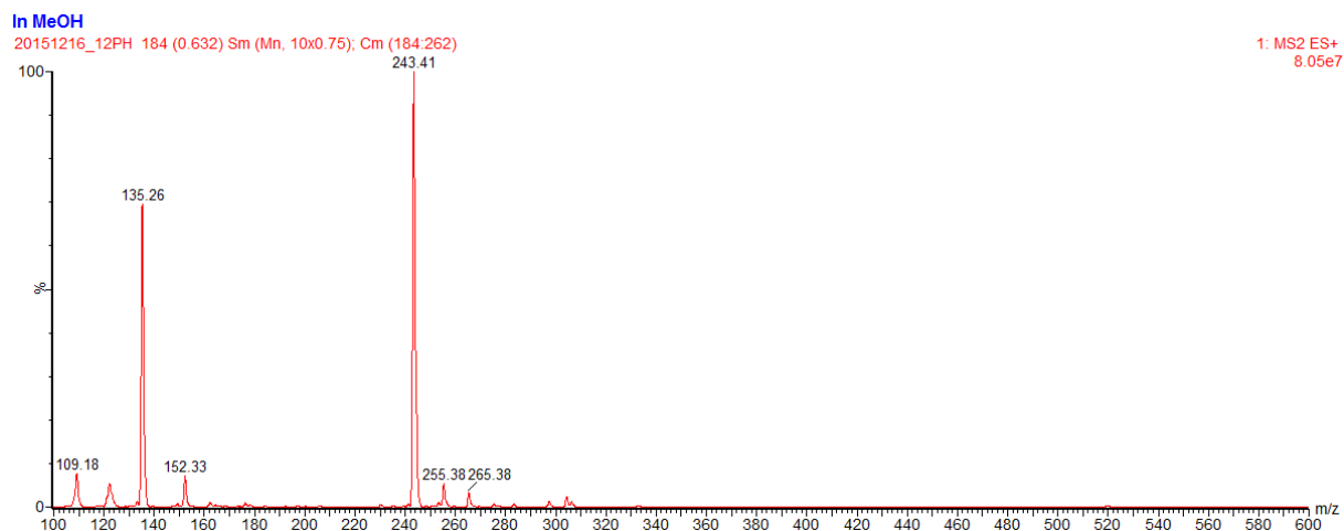
Figure S68: ESI-MS spectra of diamine N,N' -bis(pyridylmethyl)-1,2-diaminoethane picen ( 1 ).
