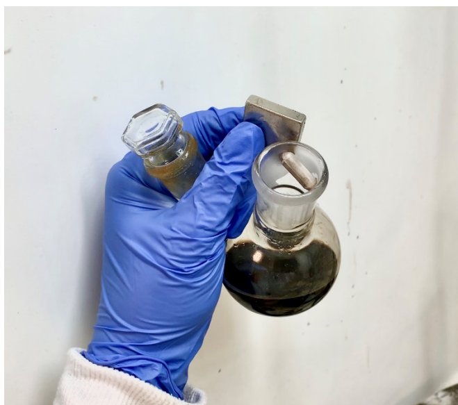
Figure S1b: (left) A demonstration of how the magnet is removed, using a second externally placed magnet. As the magnet is sitting in a position similar to the one indicated above, a solution of toluene/hexane is squirted onto the magnet, to remove nanoparticles that adhere to the magnet. (right) Typical example of the appearance of nanoparticles after centrifugation following their second wash. The supernatant will be a straw yellow colour.
