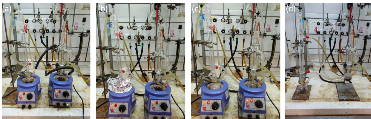
Figure S1a: Reaction set up using a gas manifold where (a) illustrates a simple degassing procedure; (b) foiling/stoppering of flask prior to reaction; (c) end of reaction, foil has been removed for clarity; (d) flasks are totally removed from mantles for cooling.
