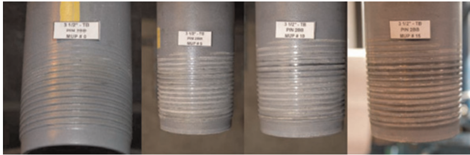
Fig. 2. Condition of Dopeless pins after 5, 10, 15 M&B cycles.
