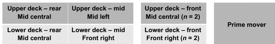
**Fig. 1.** Stylised plan of the upper- and lower-deck compartments of the B-double truck (not to scale), and the placement of the loggers. All Hobo loggers were placed at or slightly above head height of the steers, in positions to remain untouched by the steers.
