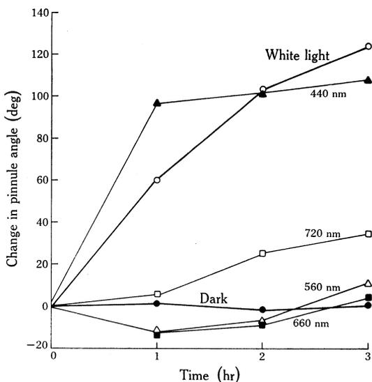
Fig. 4.—Change in pinnule angle with time at four stations on the spectrograph—440, 560, 660, and 720 nm, and also under intense white light and in darkness. Flux density at the spectrograph stations was  $0.78 \times 10^{15}$  quanta  $\text{cm}^{-2} \text{s}^{-1}$ .
