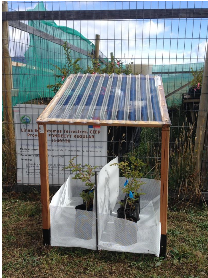
Fig. S1. Rain exclusion roof at the start of the experiment in February 2018. One sapling per each of four species were subjected to drought, whereas another four were well-watered over the experiment and considered as controls. Notice the net separating the groups of control and drought-subjected saplings, which was done to avoid the mixing of litter between watering treatments.
