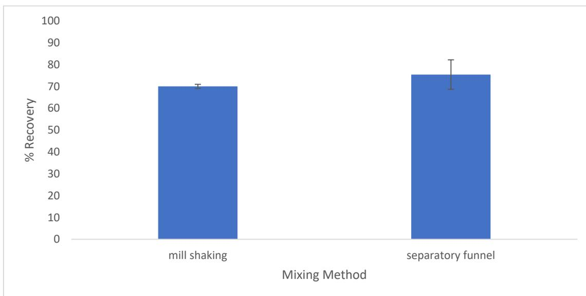
**Figure 7:** Comparison of the extraction efficiency and precision of ball mill shaking versus manual shaking in a separatory funnel. Error bars reflect the standard deviation of the measurement from triplicate analysis.
