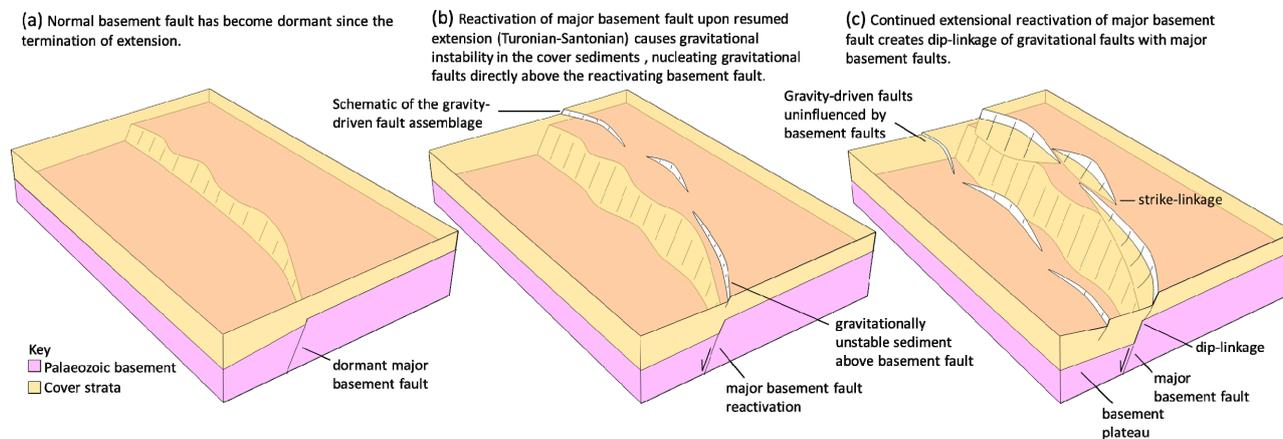
**Figure 4: Schematic diagram showing our three-stage interpretation of normal fault development. The three stages (a, b and c) are explained in the figure and text.**
