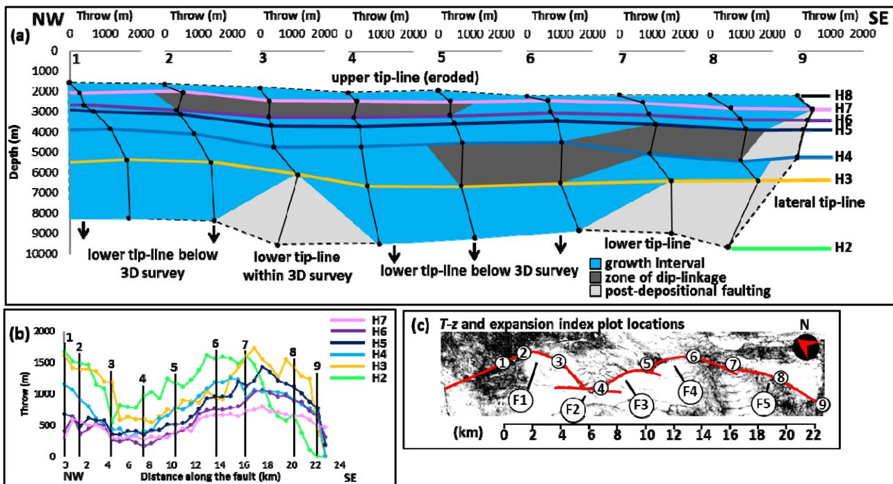
Figure 2: (a) Throw-depth ( $T-z$ ) analysis from NW (left) to SE (right) of the fault assemblage, comprised of faults 1-5. Note the upper zone of dip-linkage (dark grey) at locations 2-5 and the lower zone of dip-linkage at locations 5-8. (b) Maximum throw-distance graph showing the variability of throw along strike of the fault for horizons 2-7. The location of  $T-z$  plots 1-9 are displayed (c).
