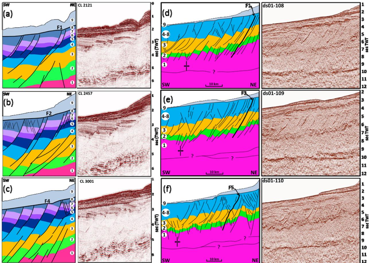
Figure 3: Crosslines 2121 (a), 2457 (b) and 3001 (c) of Amrit 3D with interpretation on the left hand side (See Figure 1 for location of crosslines). Regional 2D seismic lines ds01-108, ds01-109 and ds01-110 used to show the linkage of the fault assemblage to major basement faults. The numbers on the right hand side of all interpreted cross-sections represent stratal units we used for this study (see methods).
