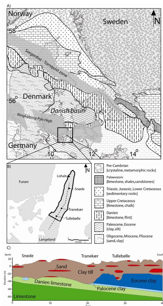
**Figure 1:** A) Overview map showing the geological setting in the Danish basin. B) The study area (marked with black). C) Conceptual geological profile through the northern part of Langeland. The position of the profile is shown as the dotted line on B.
