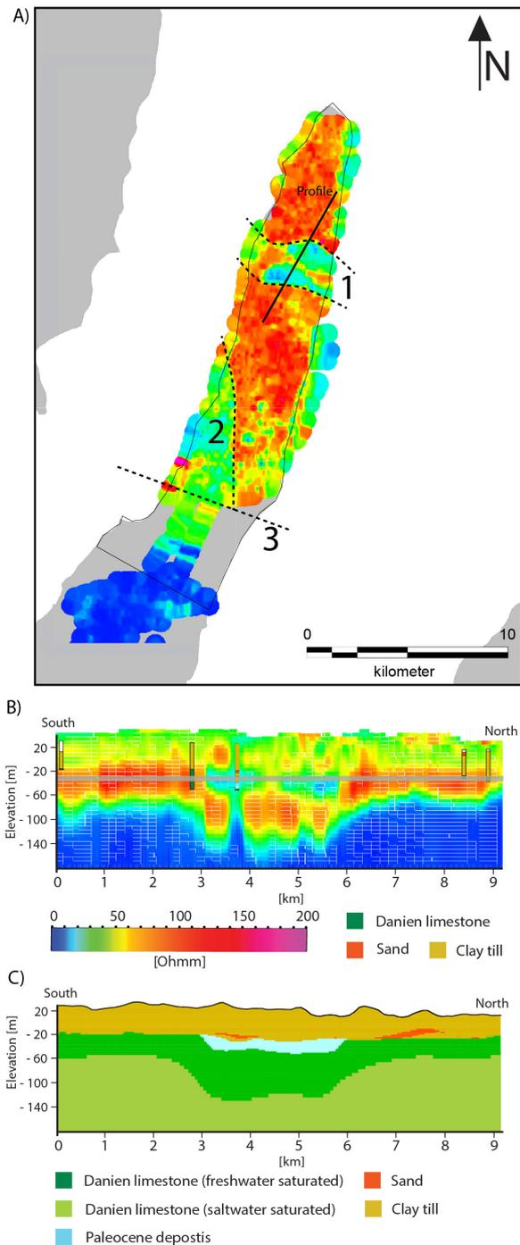
**Figure 3: A) Mean resistivity map at the elevation -25 m. B) Cross section through the northern fault system with the presence of AEM data and boreholes. The elevation of the mean resistivity map is shown with the grey line. C) Interpreted geological model**
