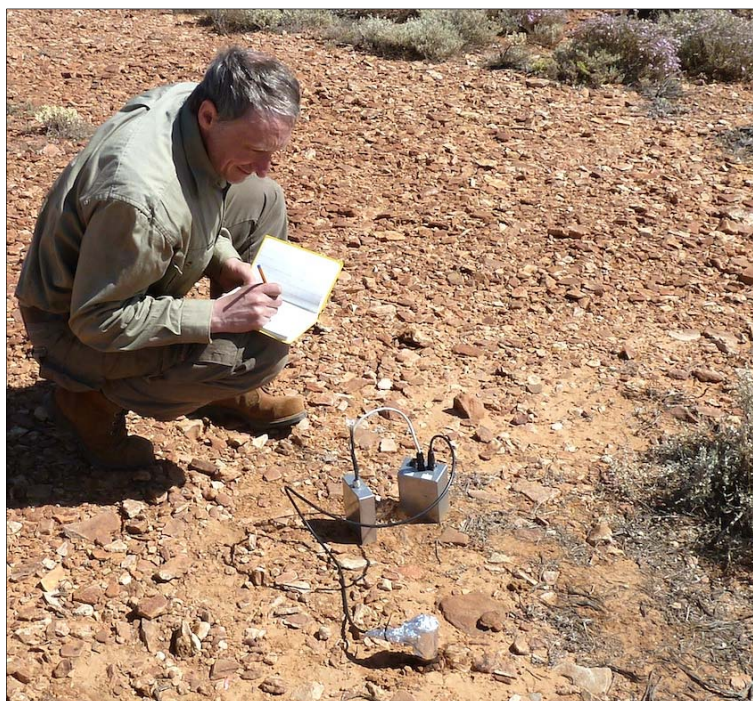
Figure 4: The author field trialling a shallow heat flow probe in South Australia in 2012.
