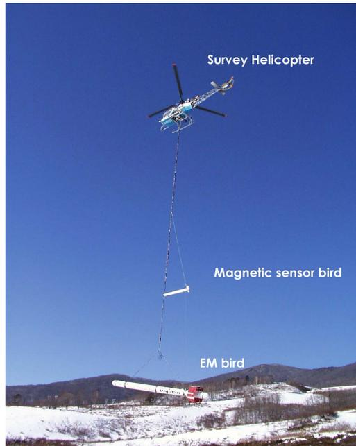
**Photo 1** Picture of the survey helicopter (SA315B) used for the airborne EM and magnetic survey over Iwate volcano (Okuma et al., 2008). Birds for magnetics and EM were suspended from the helicopter
