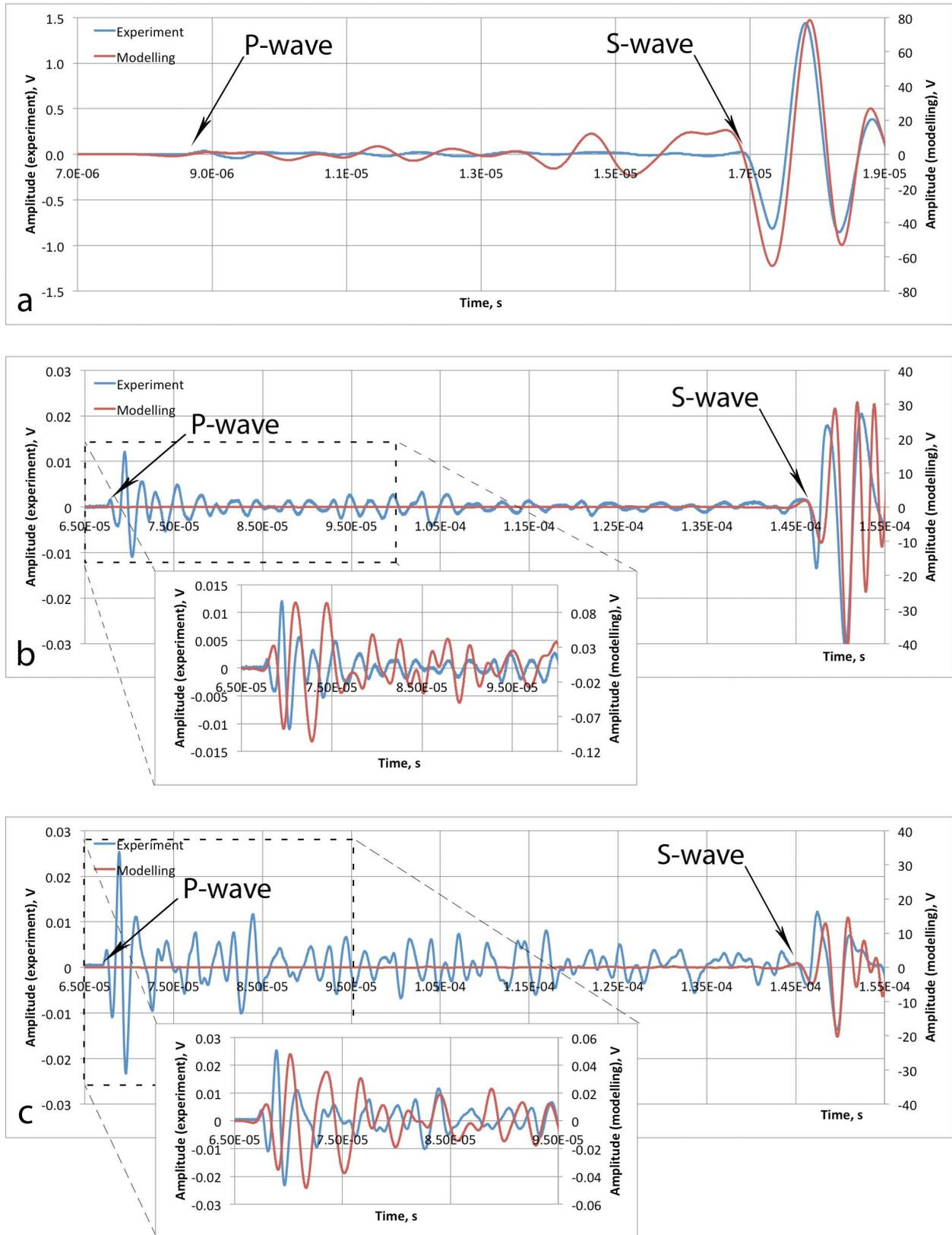
Figure 5: Simulated and experimentally obtained waveforms from receiver for three set-up configurations: a) solid aluminum cylinder; b) PMMA between two PEEK cylinders; c) aluminum disc with PMMA between two PEEK cylinders.
