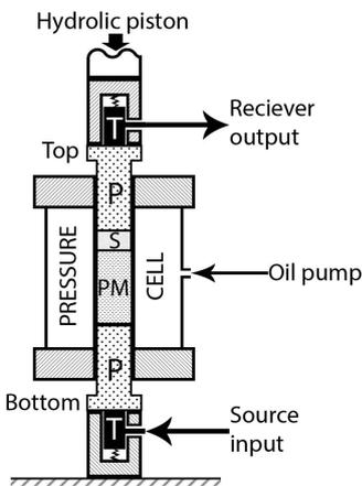
Figure 1: Scheme of pressure cell and experimental set-up. T – transducers, P – PEEK cylinder, PM – PMMA, S – sample.
