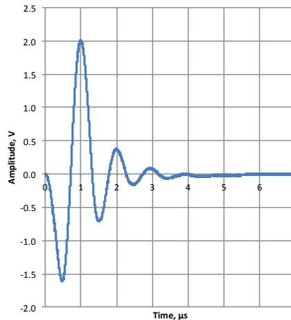
Figure 2: Recorded signal. Source and receiver transducers are in direct contact.
