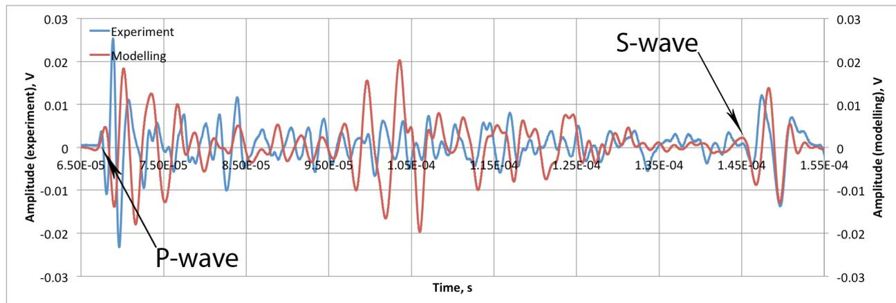
**Figure 6: Waveforms obtained for PEEK / PMMA / aluminum disc / PEEK set-up. Comparison of experimentally obtained waveform and simulated waveform with exponential dissipation of amplitude.**
