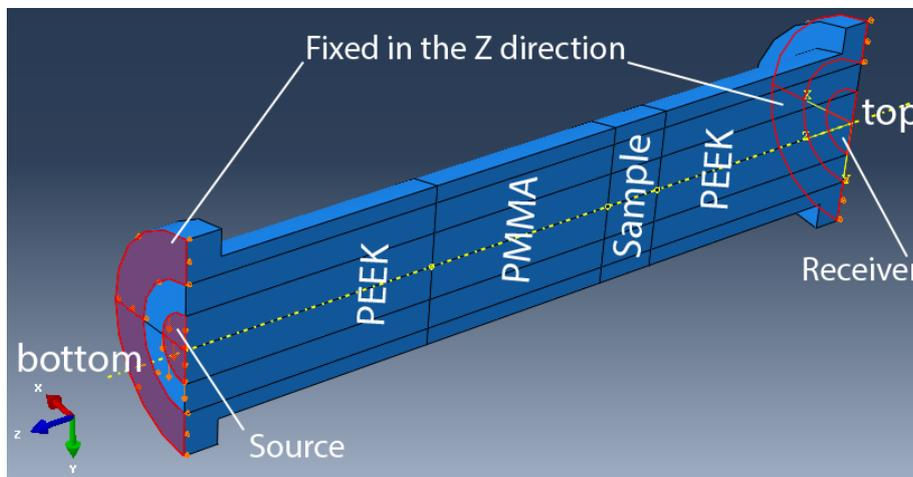
Figure 3: Computational domain with highlighted regions of fixed area, source and receiver. Boundary conditions are applied to YZ plane to introduce symmetry in the X direction.
