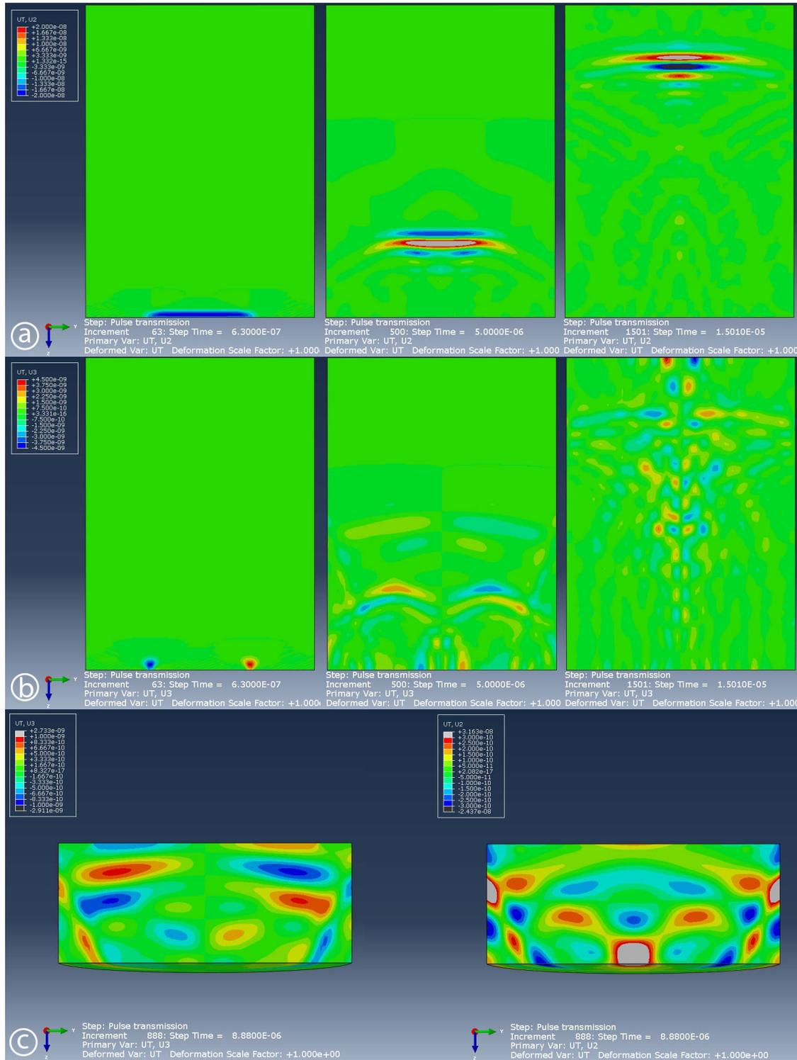
Figure 4: Simulated wave propagation in solid aluminum cylinder. a) Displacement of particles in the Y direction (U2); b) displacement of particles in the Z direction (U3), initiation and propagation of the compressional dipole; c) top part of the domain, left – U3, right – U2 at the same moment of time.
