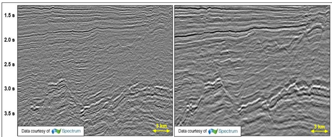
Figure 6: Crossline comparison between the legacy PSTM time stack (left) and the PSDM stack stretched to time (right)
