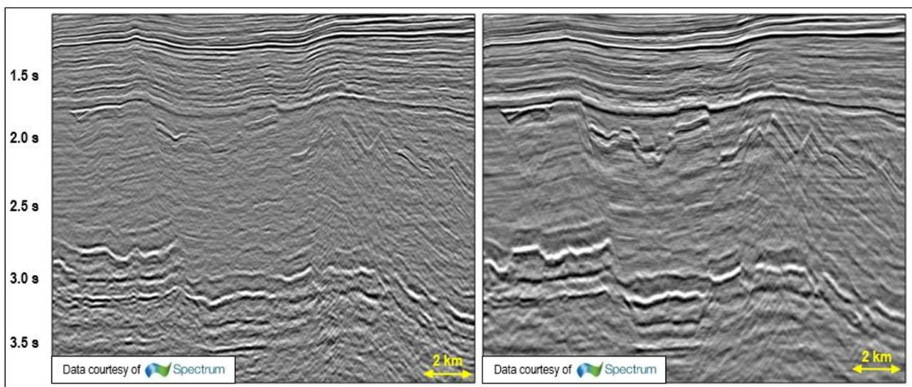
Figure 5: Inline comparison between the legacy PSTM time stack (left) and the PSDM stack stretched to time (right)
