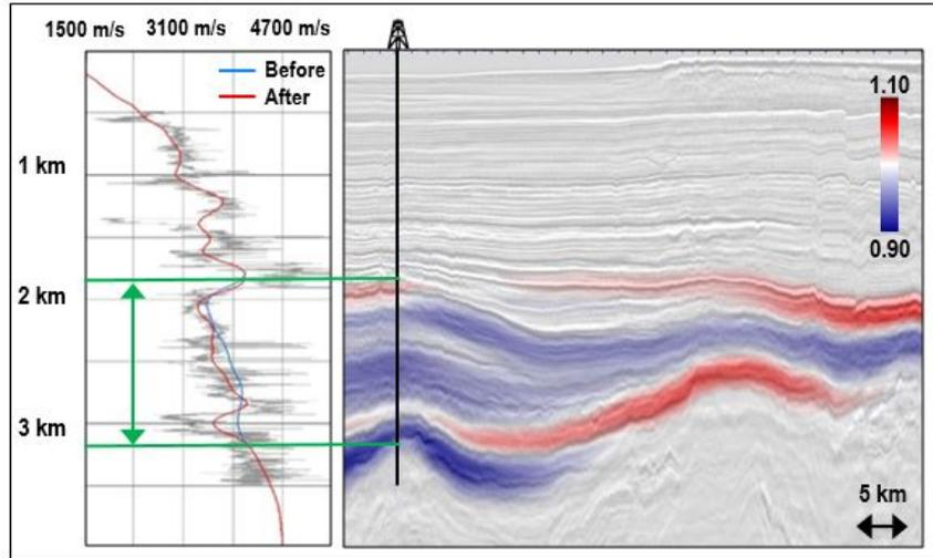
**Figure 3 Residual well velocity correction shown at a well location (left) and as a 3D scalar model (right)**
