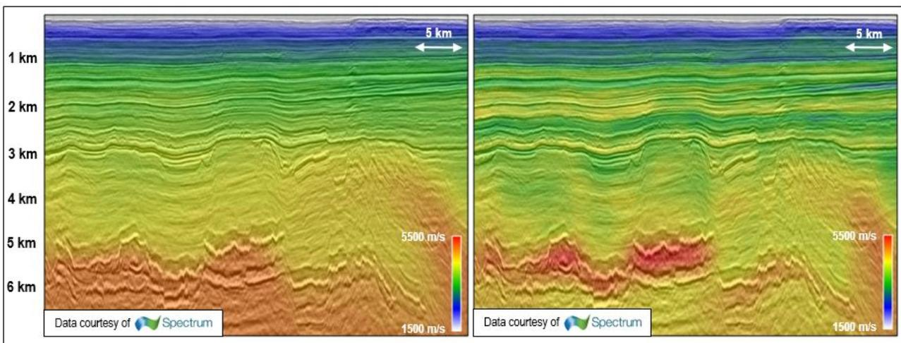
**Figure 4: Initial velocity model (left) compared to the final velocity model (right)**
