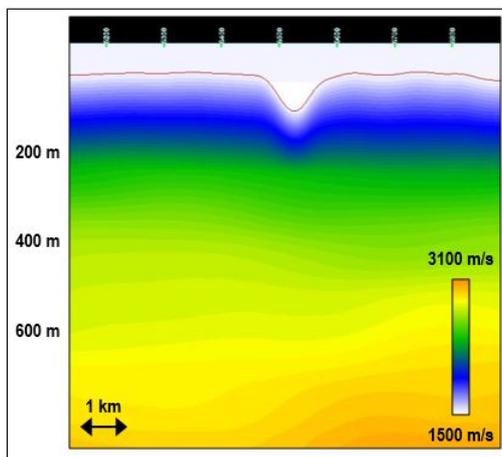
**Figure 2: Estimated velocity model beneath the seabed canyon, with the seabed position illustrated by the red line**
