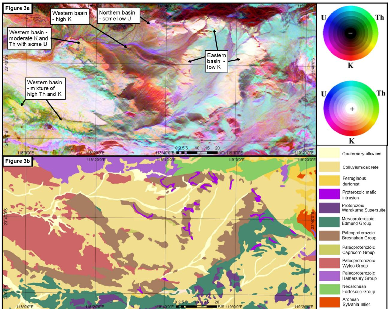
Figure 3: Highlights the radiogenic proportion differences across the basin, in particular the highly variable components in the western portion of the basin, Fig. 3a, a gamma ray coloured image showing the proportions of U, Th and radiogenic K, Fig. 3b, the surface geology for the region.
