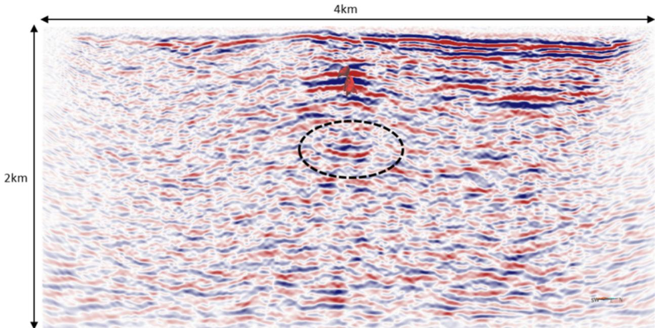
**Figure 4** Depth converted seismic image from Line 3. The wireframe of the K44 orebody is overlain on the centre top of the image. A zone of anomalous reflectivity within the host fault zone is highlighted by the dashed black oval beneath this at approximately 1km depth.
