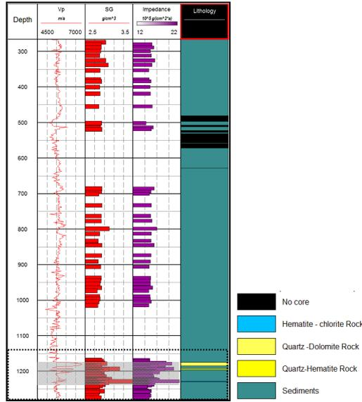
Figure 2 Plot showing the FWS log, core density measurements, the acoustic impedance derived from these and a simplified lithology log for GODD032. The logs show little variability except for the strong contrast associated with alteration near the base of the hole (highlighted by grey shading). The dashed box shows the extent of the zoomed area shown in Figure 3.
