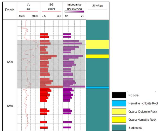
Figure 3 Zoomed in section of the results shown in Figure 2 showing more detail of the variations in seismic velocity, density and acoustic impedance associated with the quartz dolomite, quartz hematite and hematite chlorite rock near the base of the GODD032. The grey shading shows the extent of the anomalous zone highlighted in Figure 2.
