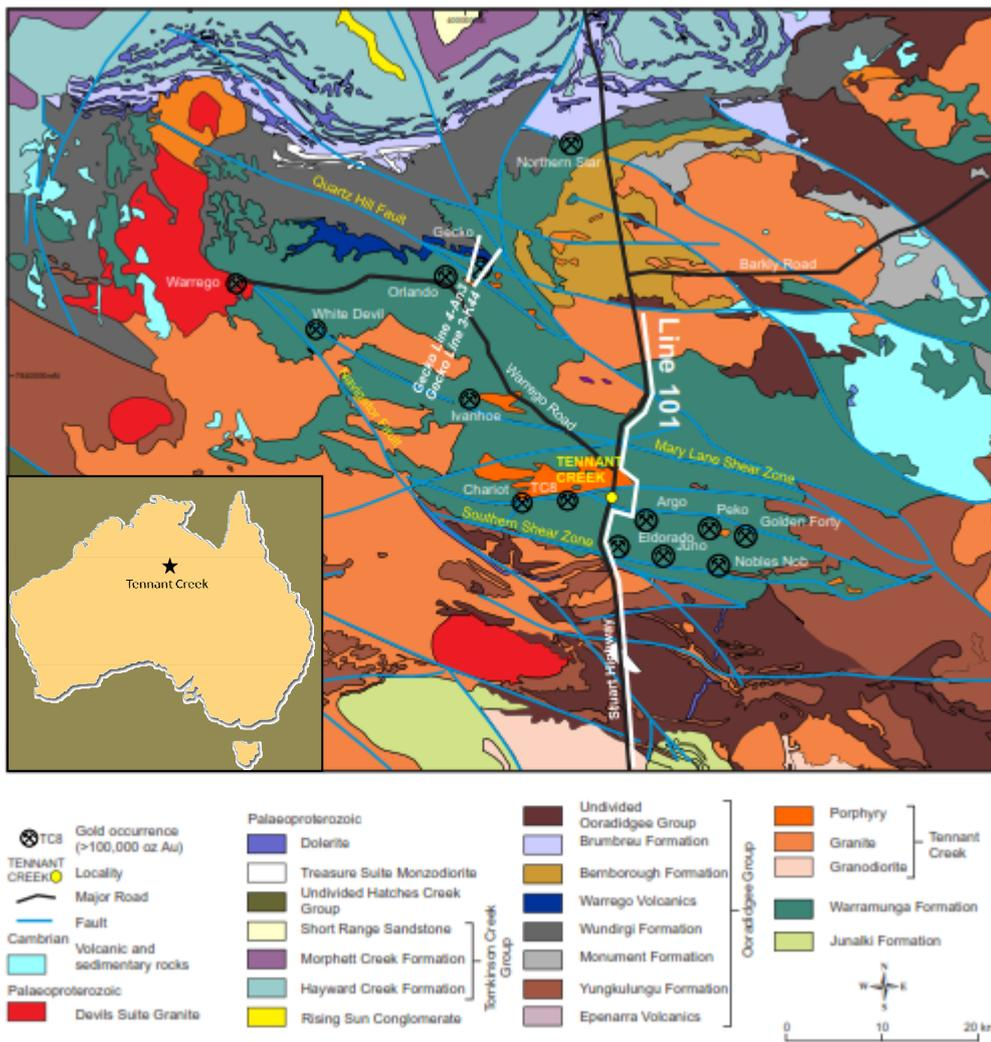
Figure 1 Location of the Gecko seismic lines (Lines 3 and 4) and the regional seismic line (Line 101) overlain on a geological map of the Tennant Creek Mineral Field
