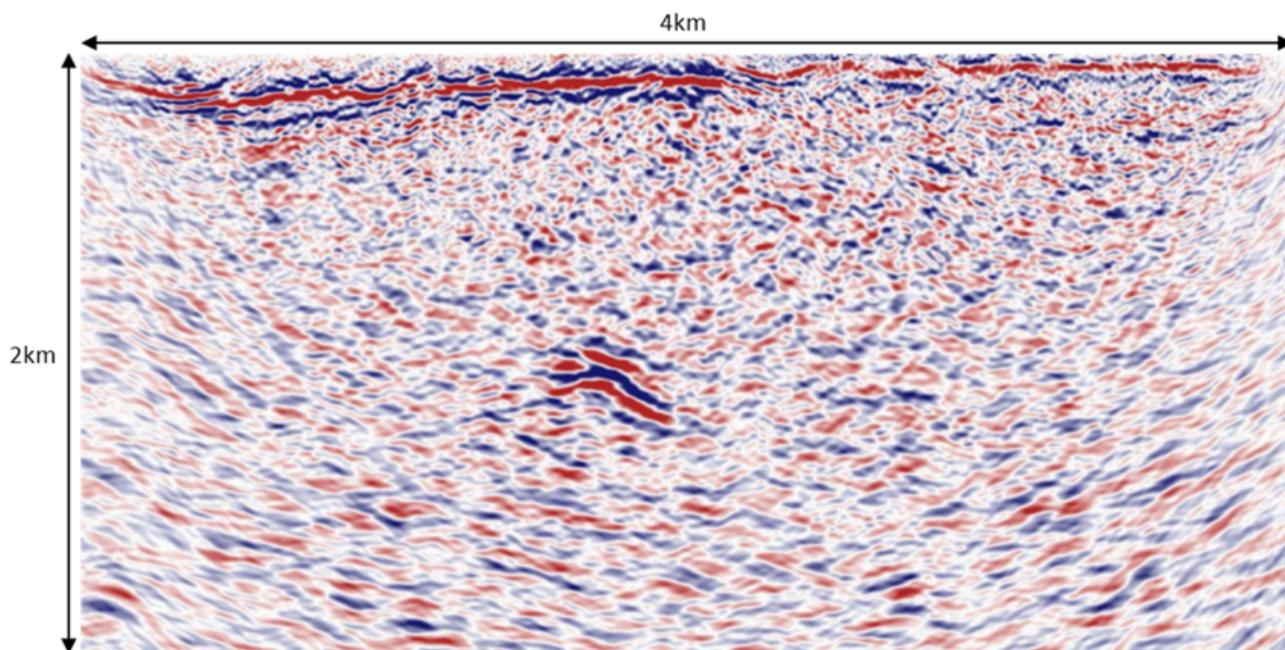
Figure 5 Seismic reflection image from Line 4. There is a distinct strong reflector at approximately 1km depth.
