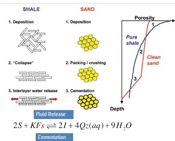
**Figure 3 Three different stages of compaction of a sedimentary basin. Channelling instabilities can occur in stage 3 at a critical overburden stress.**
