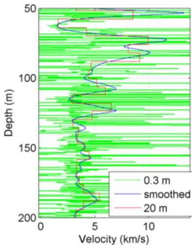
**Figure 2. Raw interval velocities (shown in green) acquired at a depth interval of 0.3 m using a tool with a sonde spacing of 15 m (Adapted from Dean et al. (2016)).**
