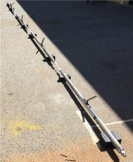
**Figure 7. String of four sondes (2 m sensor spacing), shown with the calipers fully open.**
