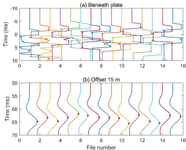
**Figure 5. Traces recorded using geophones placed (a) beneath the baseplate and (b) at an offset of 15 m. Each colour indicates a different shot. The red dots on (b) are the first break picks. The data was recorded with a sample interval of 0.25 ms.**
