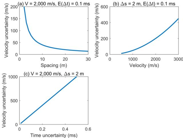
**Figure 4. (a) The uncertainty in the velocity resulting from an error in the time-pick of 0.1 ms for different depth spacing. (b) The uncertainty in the velocity resulting from an error in the time-pick of 0.1 ms given a depth interval of 2 m for different velocities. (c) The uncertainty in the velocity for a velocity of 2,000 m/s and spacing of 2 m for different time-pick errors.**
