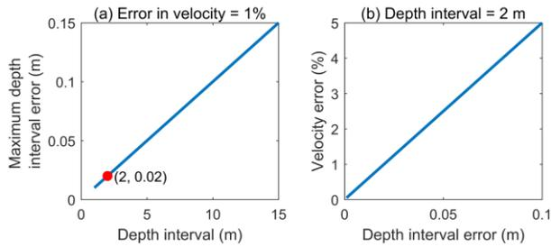
**Figure 3. (a) The maximum error in the depth interval relative to the depth interval to achieve a velocity error of 1%. (b) The error in the velocity relative to the depth interval error given a nominal depth interval of 2 m.**
