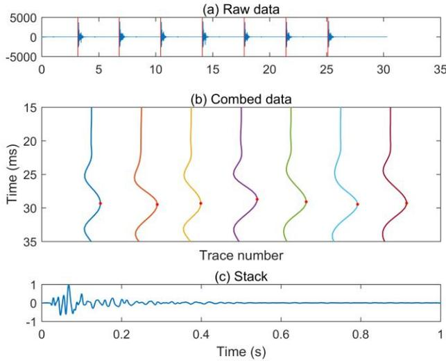
**Figure 10: (a) raw data showing six shots recorded over a 30 s period. (b) the six records removed ('combed') from the data shown in (a). (c) Resulting stacked trace.**
