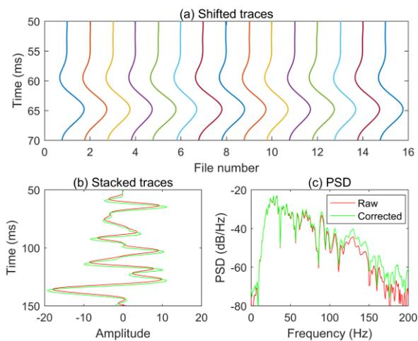
**Figure 6. (a) Traces shown in Figure 5a after trigger time variation has been removed, (b) stacked traces for the raw and time-corrected data, (c) power spectral density plots for the traces shown in (b).**
