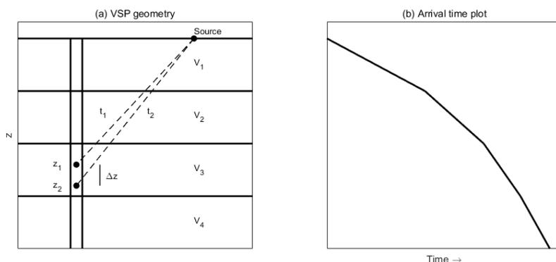
**Figure 1. (a) Diagrammatic representation of a VSP survey and (b) resulting arrival time plot.**
