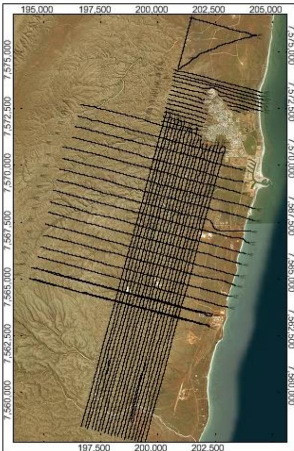
**Figure 1: SkyTEM Flight path on aerial photography.**
