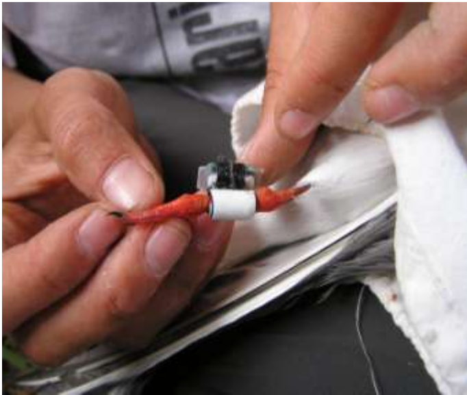
Fig. S1. Leg of a Common Tern showing a Mk10 geolocator deployed on a Darvic ring.
