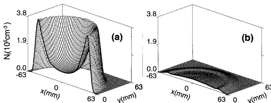
**Fig. 12.** Spatial density of the excited  $A^+(4p^4D_{7/2})$  level of the argon ion in ICP at 0.5 Torr: (a) 10 sccm flow rate and (b) 100 sccm flow rate. These data show a dramatic drop in emission at an increased flow rate due to the loss of metastables which are necessary to produce emission of the high threshold ionic line. [Reproduced from Okigawa *et al.* (1996).]
