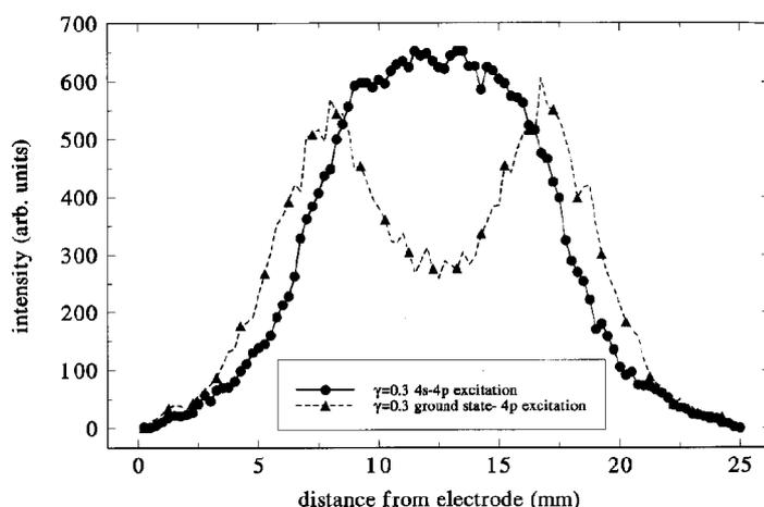
**Fig. 10.** Spatial distribution of emission in relative units for a capacitively coupled discharge in argon at 0.25 Torr at 13 MHz. The line with triangles corresponds to the direct excitation of the  $2p_1$  level, i.e. 811.5 nm emission. The line with circles corresponds to the stepwise excitation from the 4s state of the  $2p_9$  level, i.e. 750.4 nm emission.
