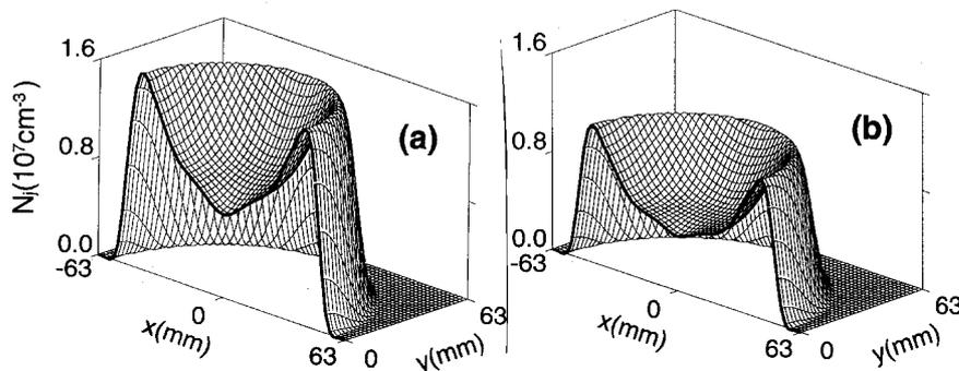
**Fig. 11.** Spatial density of the excited  $3p_5$  level of argon in ICP at 0.5 Torr: (a) 10 sccm flow rate and (b) 100 sccm flow rate. [Reproduced from Okigawa *et al.* (1996).]
