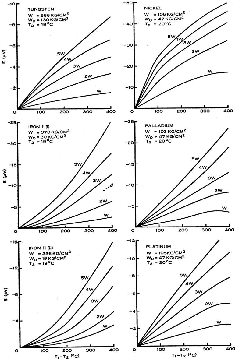
Fig. 3.—E.M.F. of strain thermocouples as a function of the temperature difference between hot and cold junctions for particular stress intensities.
