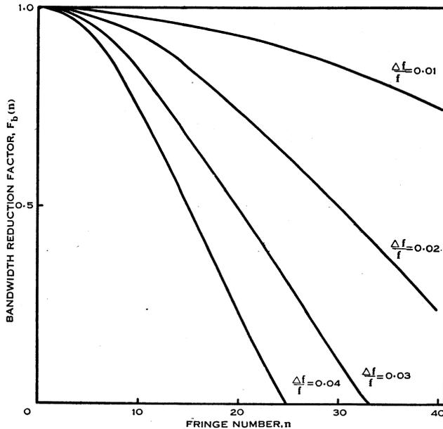
Fig. 1.—Curves showing the effect of receiver bandwidth with increasing fringe number on the amplitude of interference fringes for four ratios of bandwidth to frequency.
