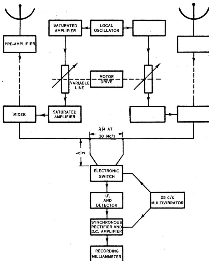
Fig. 10.—Block diagram of the units of the azimuth interferometer.
