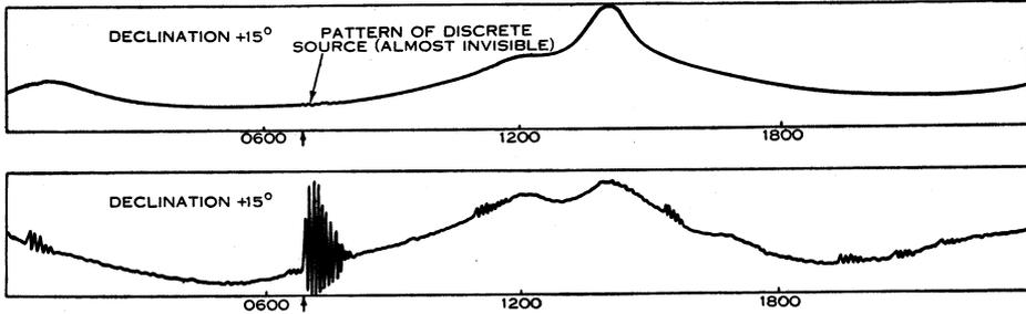
Fig. 7.—Records demonstrating the effectiveness of the automatic gain control system. The upper record is a normal total noise record and the lower is one of the same region obtained using the automatic gain control system. Note that the amplitudes of the interference patterns due to discrete sources are increased by a factor of about a hundred while the swing due to variations in the background noise is about the same.
