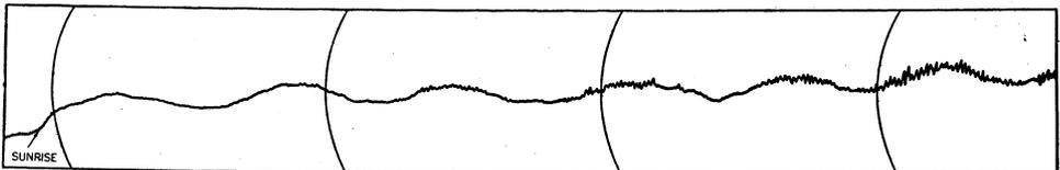
Fig. 3.—Sea interference pattern of the Sun rising showing the increasing effect of sea waves with fringe number. The curved scale lines represent intervals of 10 min. The slow sinusoidal variation is the interference pattern and the ripples are due to sea waves.
