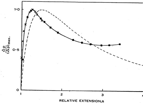
Fig. 3.—Ratio of excess pressure to its maximum value as a function of relative extension  $n$ . Squares are experimental values for a 700 g balloon, crosses for a 2000 g balloon. Dotted curve theoretical values from equation 4.  $\Delta p_{max.} = 18.3 \text{ mm H}_2\text{O}$  for 700 g,  $7.9 \text{ mm H}_2\text{O}$  for 2000 g.
