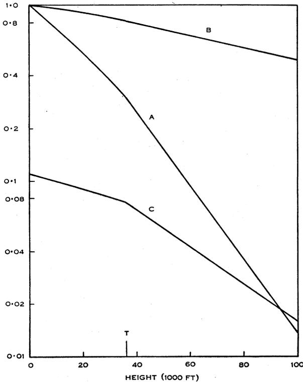
Fig. 1.—Curve *A*, density relative to ground  $\rho/\rho_0$ ; curve *B*,  $(\rho/\rho_0)^{1/6}$ ; curve *C*,  $10^{-5} RF^{-1/2}$  gram<sup>1/2</sup> ( $R$ =Reynolds number,  $F$ =free lift) plotted against height for I.C.A.N. standard atmosphere. *T* is the tropopause.
