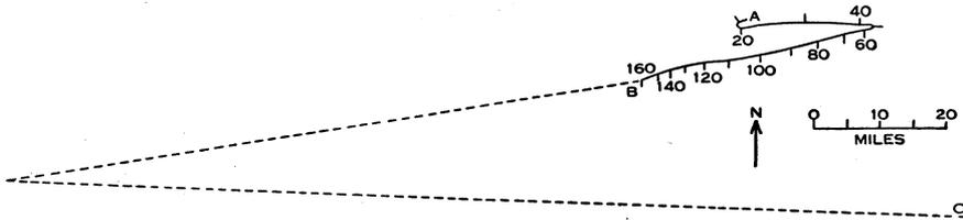
Fig. 6.—Ground projection of track of a balloon, stabilized by a valve, released at A, observed to B, and found at C. Solid curve is observed path, dotted curve path deduced from observed winds. Graduations on curve are times from release in minutes.
