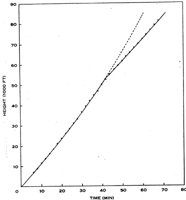
Fig. 2.—Flight of a 2000 g balloon. Solid line shows theoretical height with *k* changing by 1/0.6 at 53,500 ft; crosses are observed heights. Dotted line shows expected height if *k* does not change.
