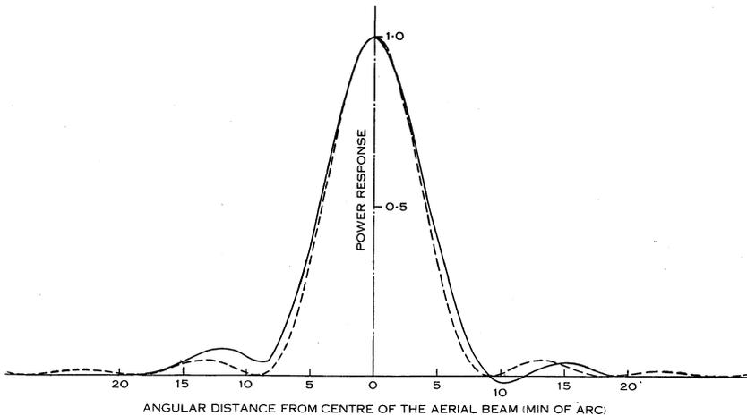
Fig. 2.—Theoretical aerial pattern (broken line) compared with the derived response of a localized bright region on the solar disk (full line).
