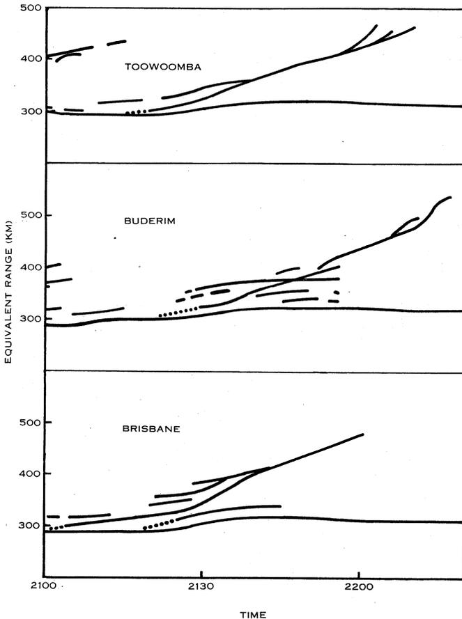
Fig. 1.—Divergent range multiplet recorded simultaneously at three separated stations. Portion of  $R't$  records for Toowoomba, Buderim, and Brisbane, July 22, 1950, replotted from readings. Some of the traces on the original records were broader than is shown and closely adjacent traces cannot be resolved from each other; the dotted portions are thus conjectural.
