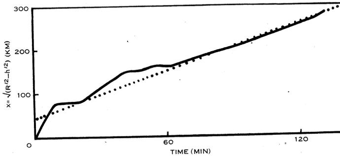
Fig. 3.—Plot of  $x(=\sqrt{R'^2-h'^2})$  versus  $t$ . (Brisbane, October 16, 1954.) The full curve joins the points plotted, the broken curve is the best-fitting straight line. Note that since  $dx/dR'$  becomes infinite as  $x$  approaches zero, the lower part of the curve is subject to great error.
