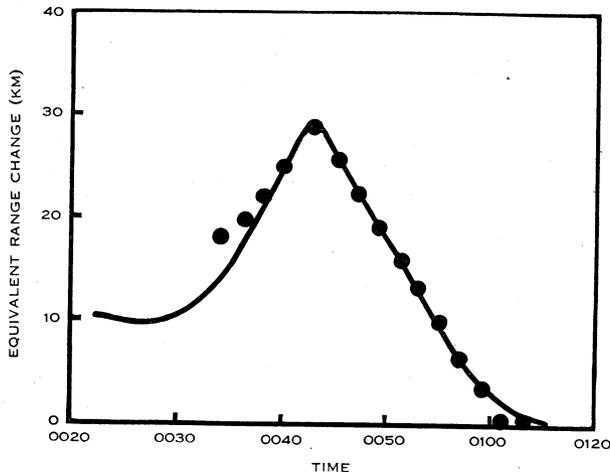
Fig. 6.—Comparison of group-path and phase-path changes. Changes of group path (full line) and phase path (dots) for lowest ("main") trace of a mixed range multiplet (June 23, 1955, at 0040 hr). The two plots have been adjusted to coincide at the peak.
