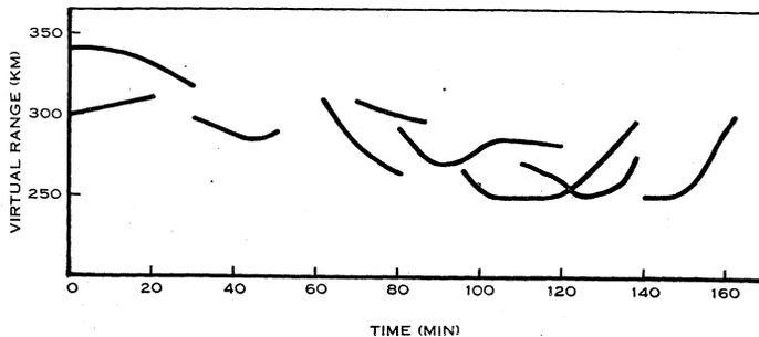
Fig. 11.—Absence of continuous main  $F$ -region trace. Replot of portion of  $R't$  record for Brisbane, Oct. 21–22, 1954. Strong  $E_s$  reflections were present but have not been plotted.
