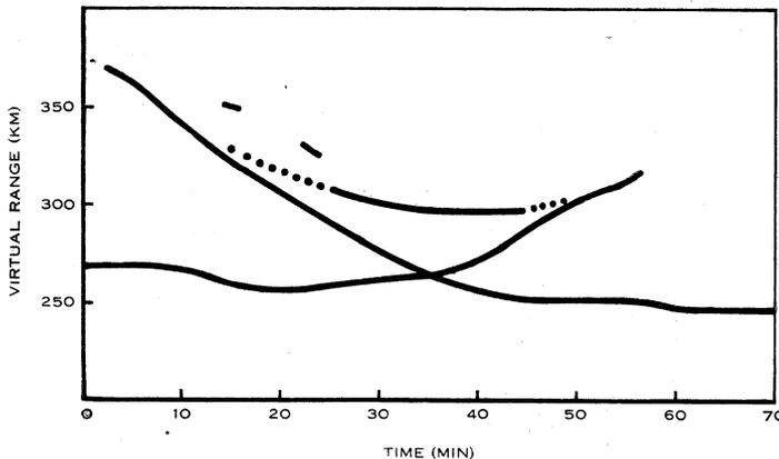
Fig. 8.—Mixed range multiplet showing traces of upper member  $R't$  record for Brisbane, March 17, 1953, replotted from readings. The dotted portions are conjectural, since the lower trace was broader than the diagram suggests and these portions of the upper satellite, if present as indicated, would have been obscured.
