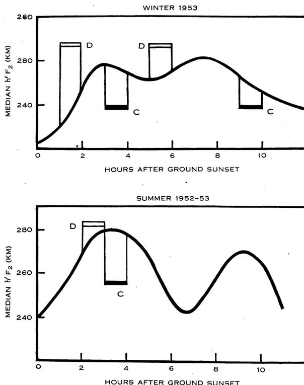
Fig. 25.—Diurnal variation of  $h'F$  at Brisbane. Upper curve winter, 1953; lower curve, summer, 1952-53. Symbols attached indicate the positions of maximum frequency of occurrence of range doublets, open rectangles indicating divergent and filled-in rectangles convergent doublets.
