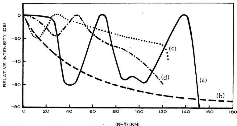
Fig. 13.—Changes of intensity (in dB) of satellite plotted against excess of range over minimum. Curve (a) represents a case of extreme fluctuation; curve (b) a case of unusually uniform change. Curves (c) and (d) represent more usual behaviour.
