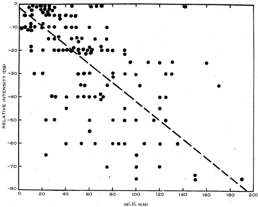
Fig. 14.—Relative intensity *v.* excess of range over minimum for satellites. Intensity taken as 0 dB at zero range excess. The broken line has a slope of  $-0.4$  dB/km.
