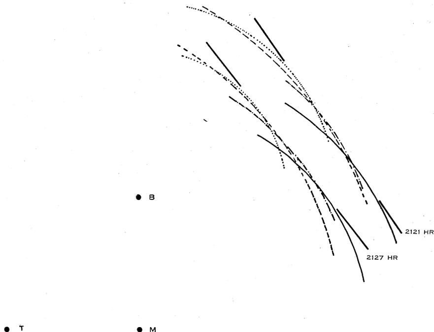
Fig. 18.—Plan of stations, with circles drawn to indicate simultaneous values of  $x = \sqrt{R^2 - h^2}$  for a satellite observed at three stations—Brisbane ( $M$ ), Toowoomba ( $T$ ), and Buderim ( $B$ ), June 23, 1955. Full lines for Brisbane; broken lines for Toowoomba; dotted lines for Buderim. The “dot-dash” line is the ellipse deduced from  $TR'$  observations (2121 hr Buderim to Brisbane, 2127 hr Toowoomba to Brisbane). The straight lines indicate the common tangent in each case.
