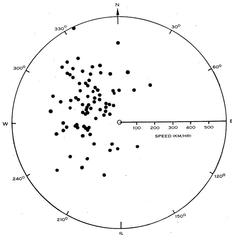
Fig. 19.—Polar plot indicating speed and directions of movement of the common tangent to the circles on the plan-position diagrams.
