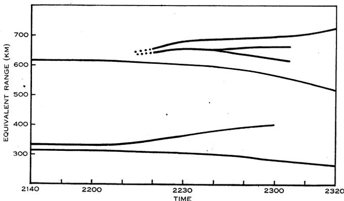
Fig. 15.—Re-plot of portion of  $R't$  records of Brisbane, Oct. 27, 1952, 2.28 Mc/s showing two (at times three) satellites on the double-hop trace.
