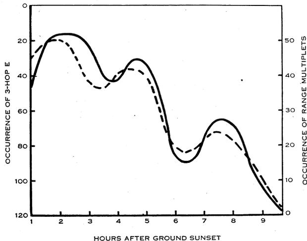
Fig. 26.—Inverse correlation between occurrence of range multiplets and  $3E_s$  reflections. Diurnal variation of occurrence of three-hop  $E_s$ , determined by number of 6-min periods for which it was present (full curve, plotted downwards). The broken curve gives frequency of occurrence of range multiplets (plotted upwards).
