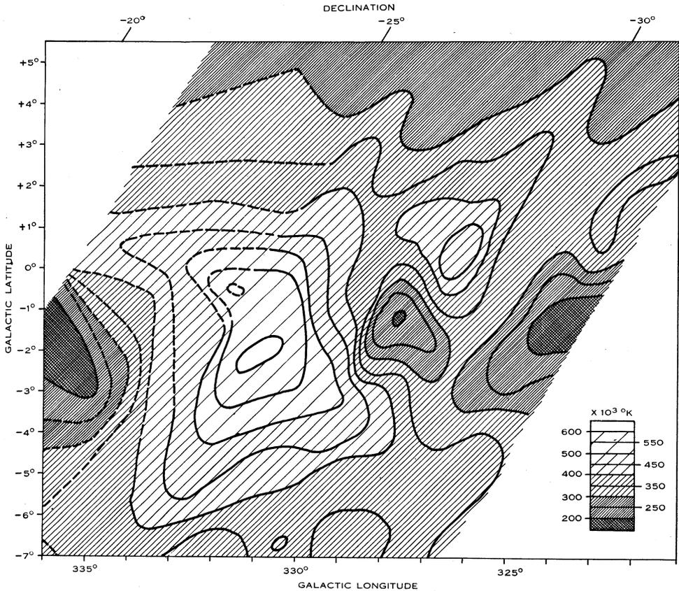
Fig. 2.—Isophotes of 19.7 Mc/s observed brightness temperatures near the galactic centre. The temperature scale is indicated by shading according to the key in the lower right-hand corner. The dark region near the centre is the source Sagittarius-A observed in absorption. The contours are dashed near the left-hand side where there were insufficient observations to give the full detail.
