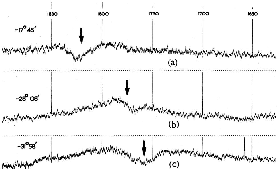
Fig. 1.—Typical records at three declinations as indicated. Sidereal time is marked and the arrows show the time at which galactic latitude  $-1^{\circ}.3$  passed the aerial beam on each occasion.
